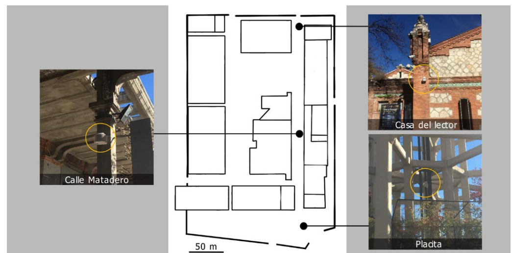
Figure 2. Locations of the three sensors (indicated with a yellow circle) installed in the outside ambits of Matadero Madrid, compiled by the authors.
