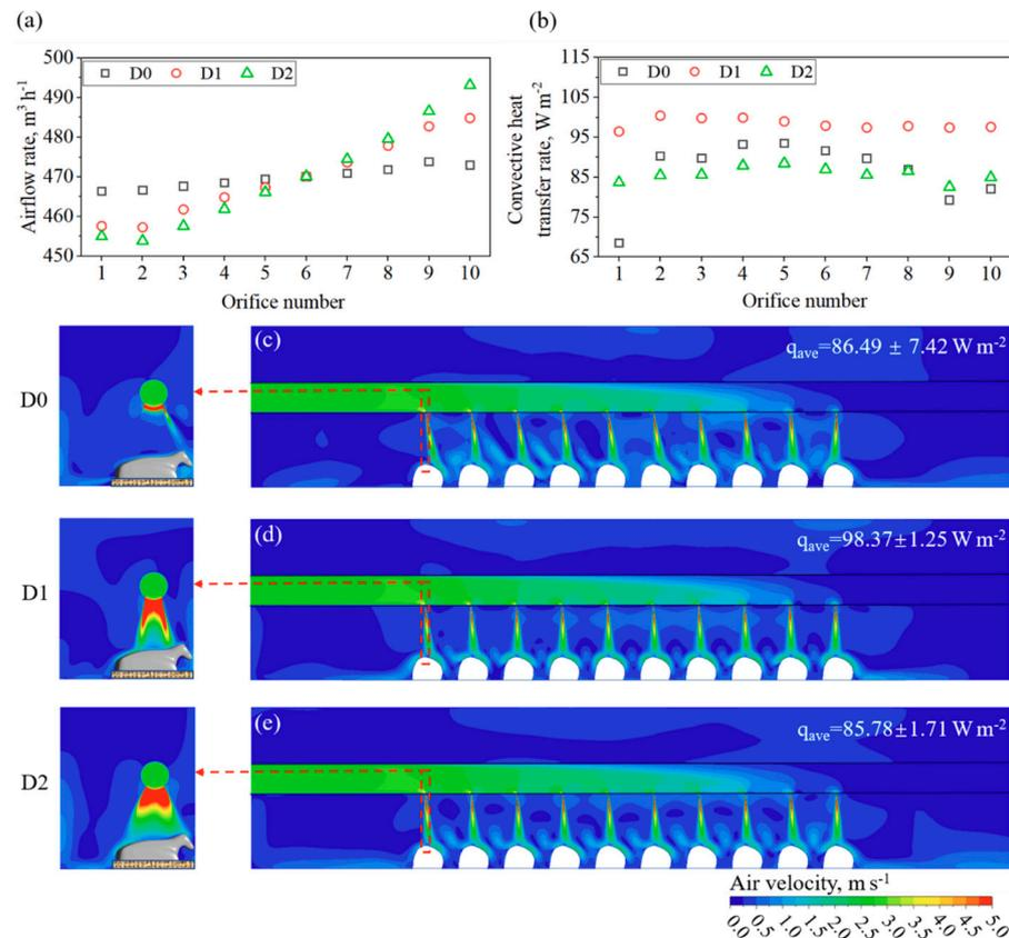
**Figure 4.** The airflow rates (a) and convective heat transfer rates (b) associated with the original PAD system without deflectors (D0) and with two different deflectors (D1 and D2), corresponding jet flow patterns (c–e).
