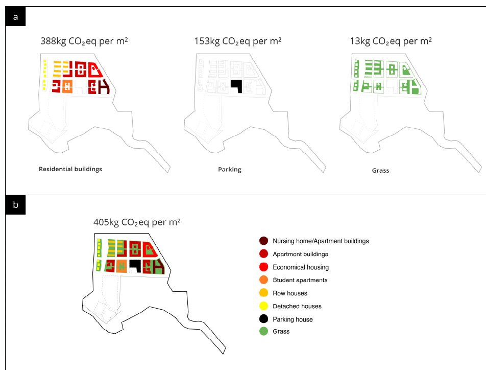
Figure 8. (a) A diagram of the results of the residential buildings, grass area, and parking house is shown separately. (b) Diagram of the results of the residential buildings, grass area, and the parking house combined together and divided by the area of the residential spaces.
