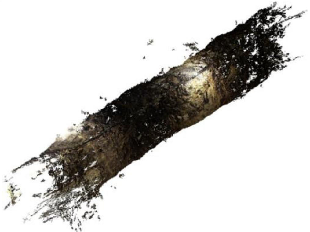
**Figure 15.** Results after dense reconstruction CMVS-PMVS.
