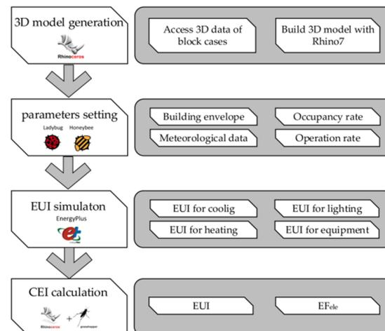
**Figure 4.** Building CE simulation based on Rhino and Grasshopper.
