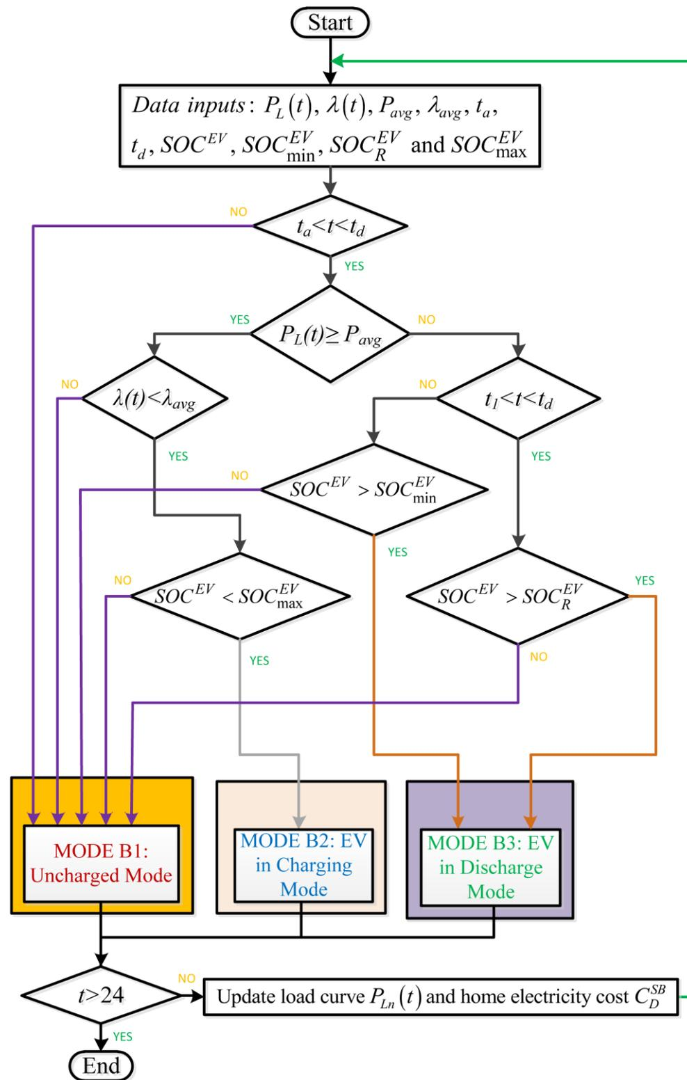
Figure 3. The energy scheduling strategy flowchart for EV charging with V2H without HESS.
