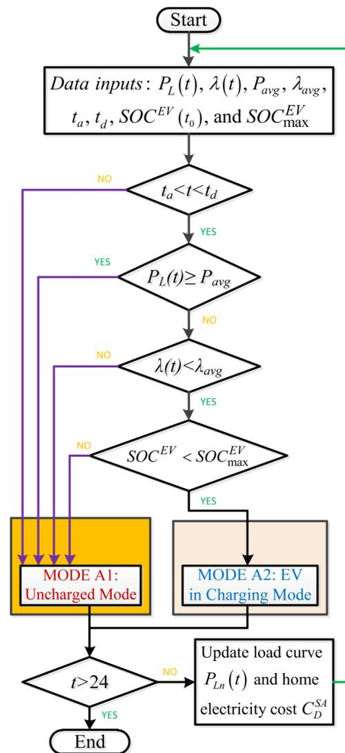
Figure 2. The energy scheduling strategy flowchart for EV charging without V2H and HESS.
