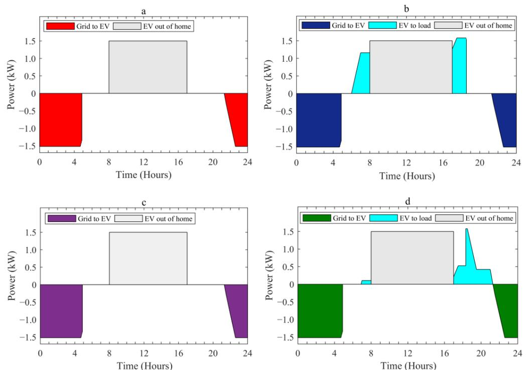
**Figure 13.** EV power curve in (a) scenario A, (b) scenario B, (c) scenario C, and (d) scenario D.
