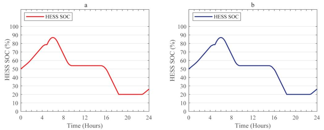
Figure 10. HESS SOC in (a) scenario C and (b) scenario D.
