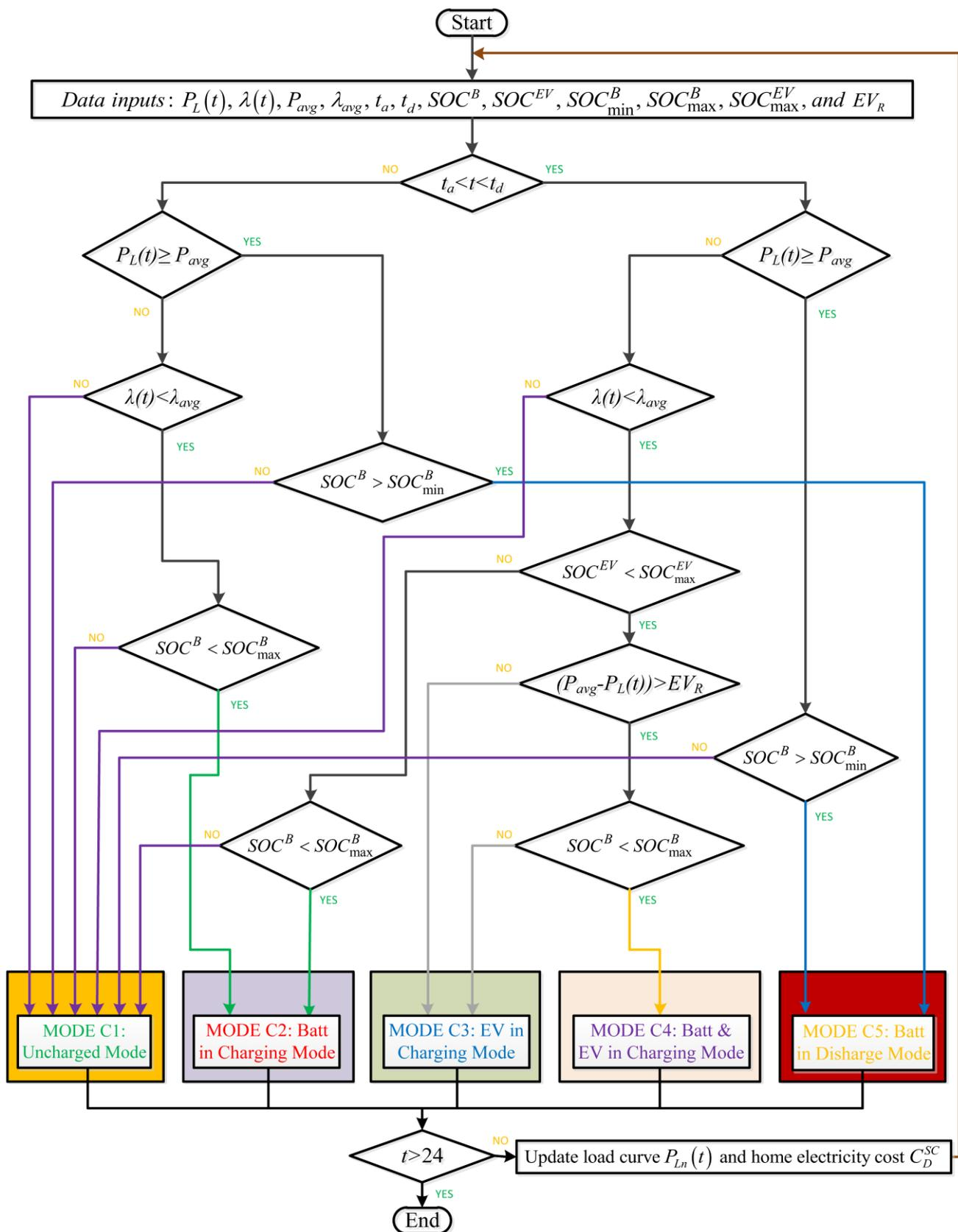
Figure 4. The energy scheduling strategy flowchart for EV charging with HESS without V2H.
