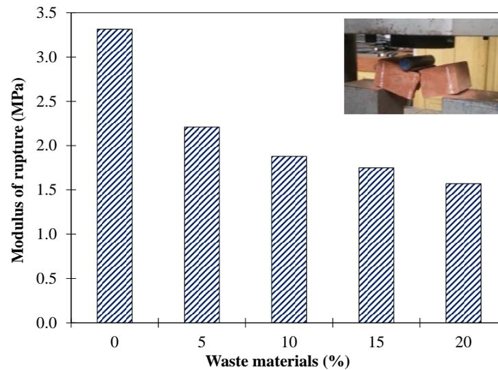
**Figure 15.** Modulus of rupture of brick specimens incorporating WMP and SBA.
