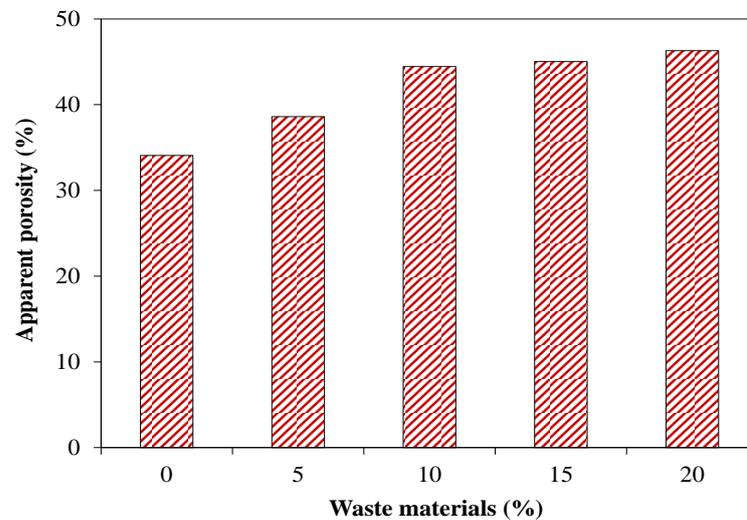
**Figure 11.** Apparent porosity for brick specimens incorporating WMP and SBA.
