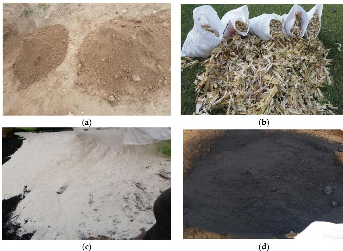
**Figure 1.** Materials used for the manufacturing of bricks. (a) Clay; (b) Sugarcane waste; (c) Waste marble powder; (d) Sugarcane bagasse ash.
