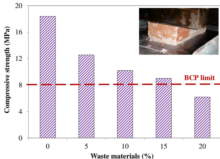
Figure 14. Compressive strength of brick specimens containing WMP and SBA.
