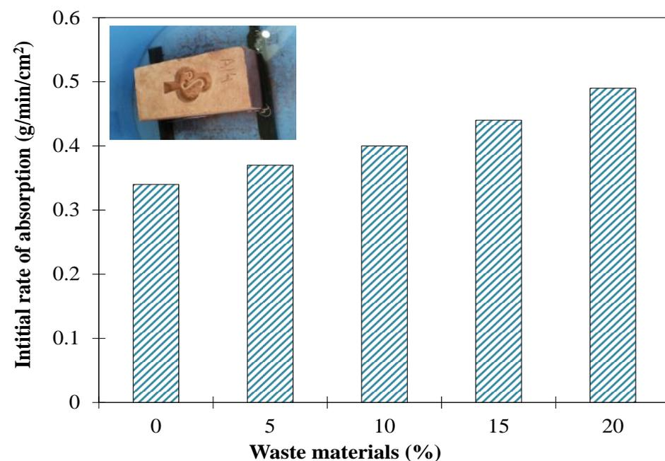
Figure 13. Initial rate of absorption for brick specimen containing WMP and SBA.
