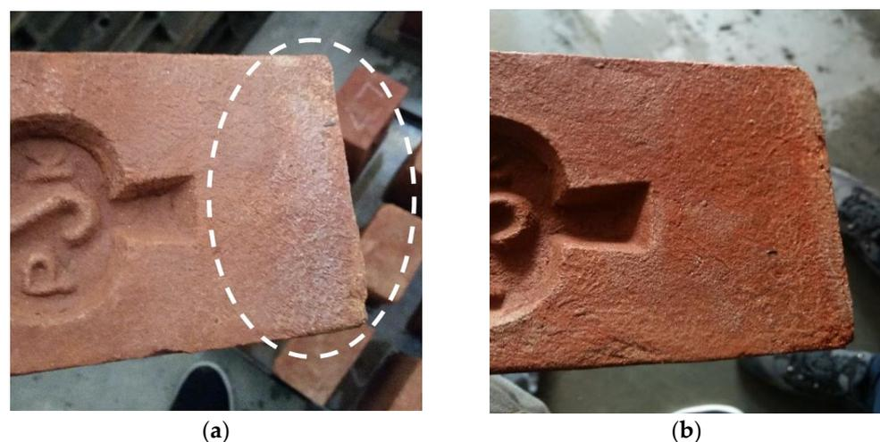
**Figure 16.** Efflorescence results after 7 days. (a) Control clay brick (slight efflorescence); (b) Brick with 5% waste materials (no signs of efflorescence).
