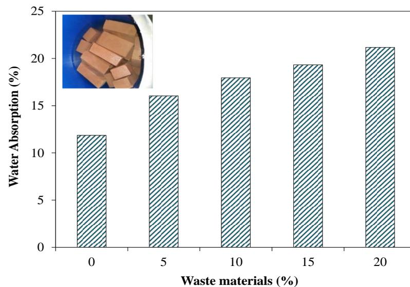
Figure 12. Water absorption of brick specimen containing WMP and SBA.
