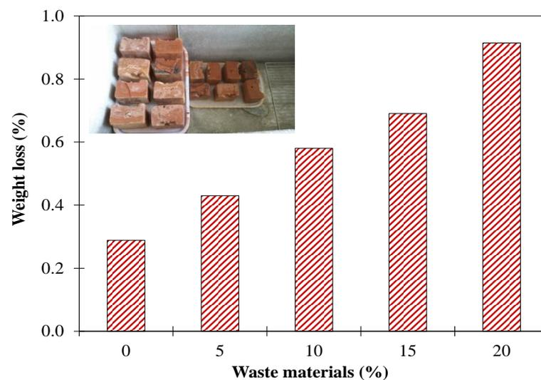
**Figure 17.** Loss of weight due to freeze-thaw.
