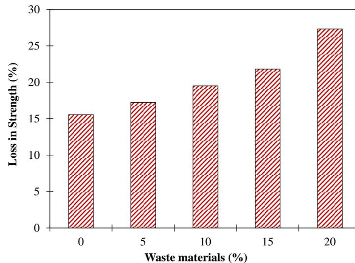
**Figure 18.** Loss in compressive strength due to sulphate attack.
