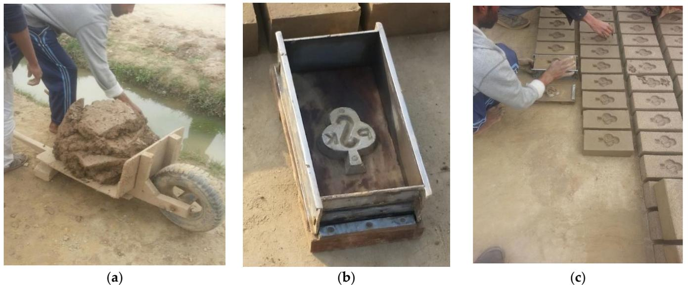
**Figure 3.** Manufacturing of brick specimens. (a) Lumps for brick manufacturing; (b) Brick mold; (c) Casting of bricks.
