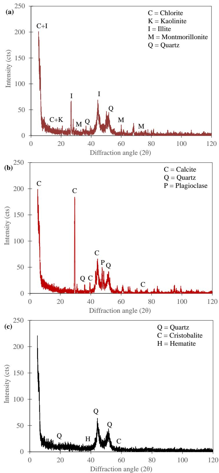
**Figure 7.** XRD patterns of used materials. (a) Clay; (b) WMP; (c) SBA.
