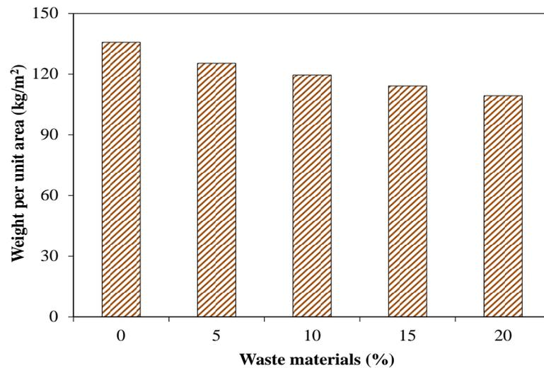
**Figure 10.** Weight per unit area for brick specimen incorporating WMP and SBA.
