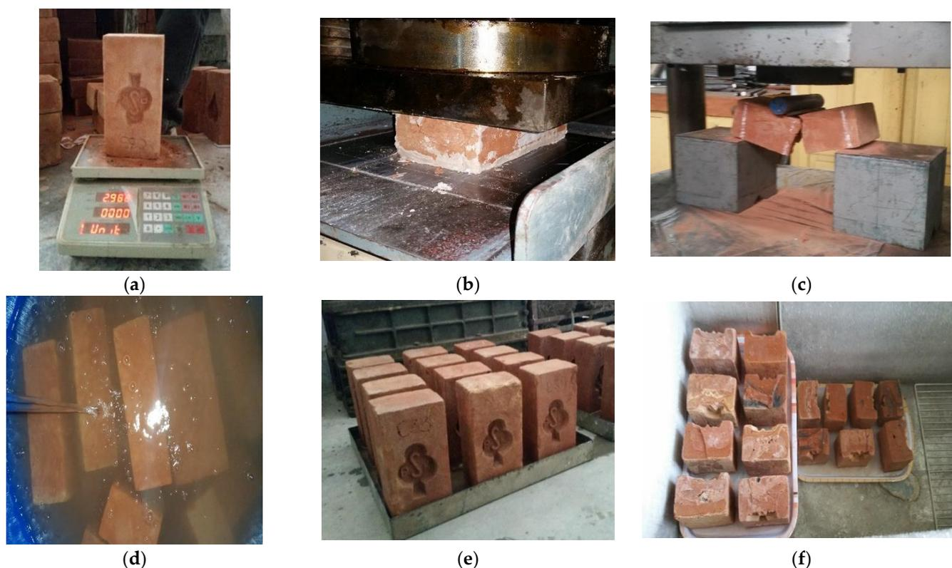
**Figure 6.** Assessment of brick specimens. (a) Unit weight; (b) Compressive strength; (c) Modulus of rupture; (d) Water absorption; (e) The specimen was placed in water for efflorescence; (f) Freeze-thaw specimens placed in cooling chamber.
