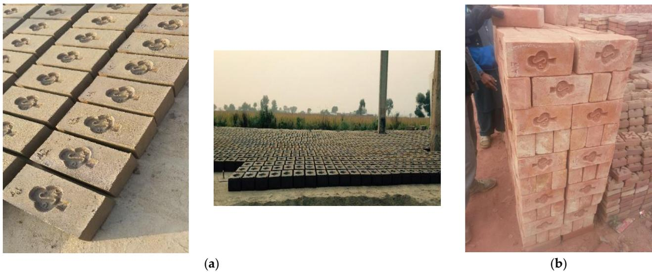
**Figure 4.** Burning of brick specimens. (a) Sun drying; (b) After burning in the kiln.
