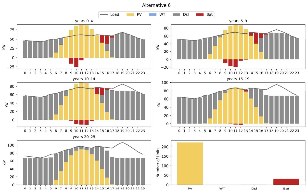
**Figure 7.** Operational scheme and number of generation units of microgrid alternative 6 in the 25 years of planning.
