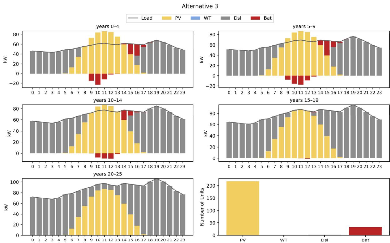
**Figure 6.** Operational scheme and number of generation units of microgrid alternative 3 in the 25 years of planning.
