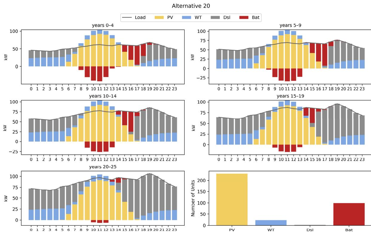
**Figure 9.** Operational scheme and number of generation units of the microgrid 20 alternative in the 25 years of planning.
