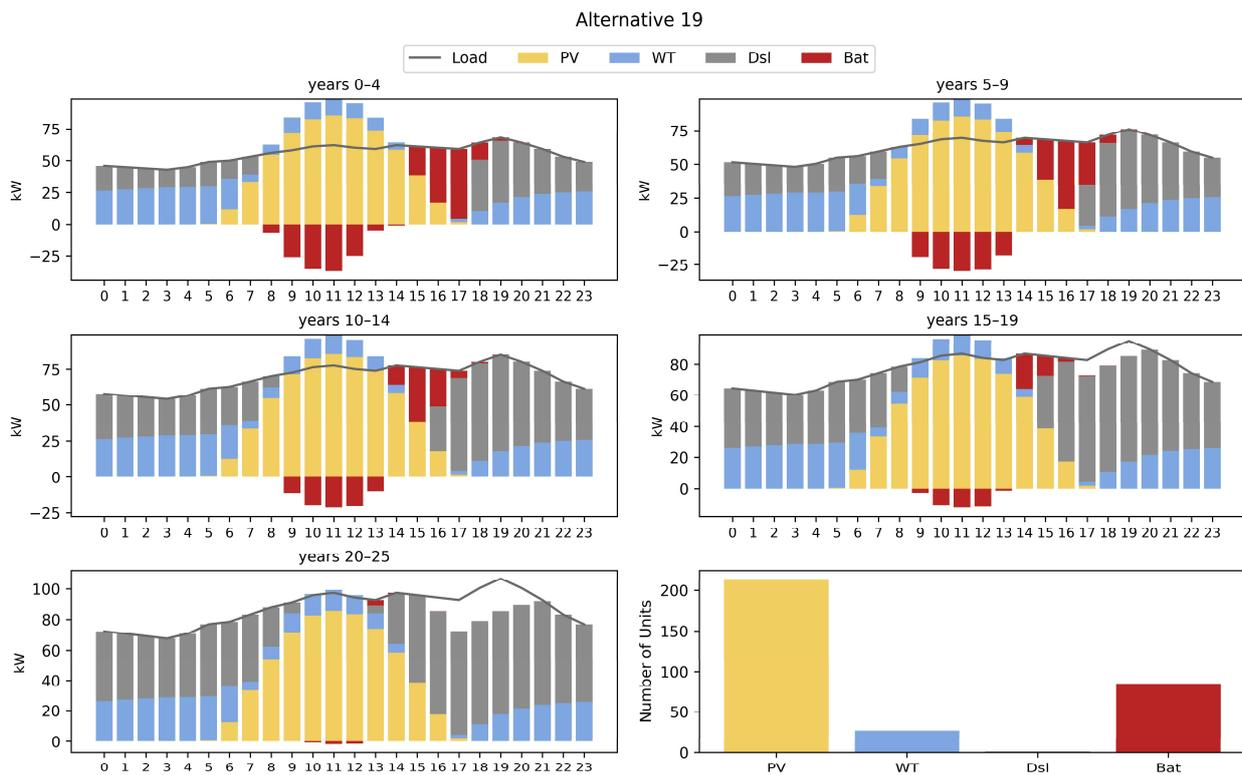
**Figure 8.** Operational scheme and number of generation units of microgrid alternative 19 in the 25-year planning period.
