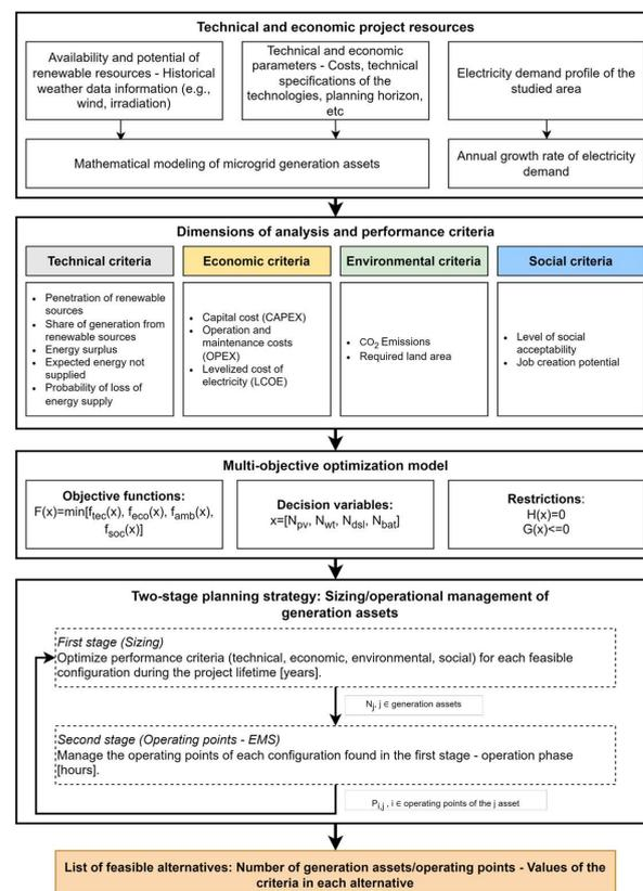
Figure 1. Framework for microgrid planning.
