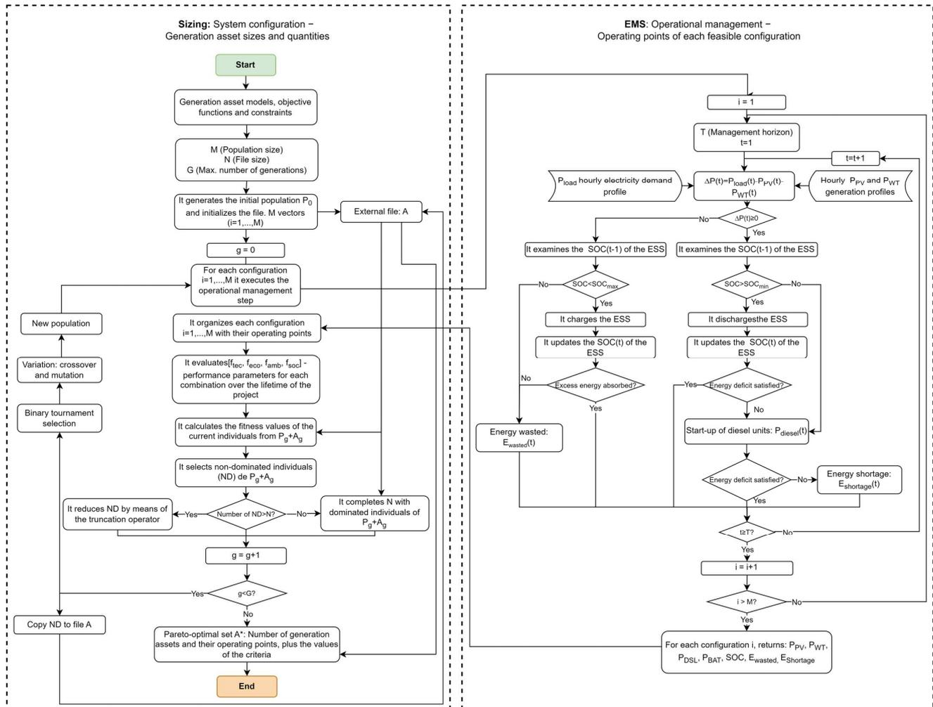
Figure 2. Two-step planning strategy for sizing and operational management of microgrid resources.
