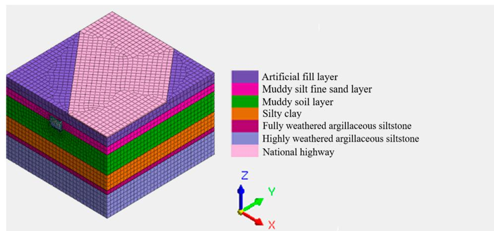
Figure 11. Numerical simulation model.
