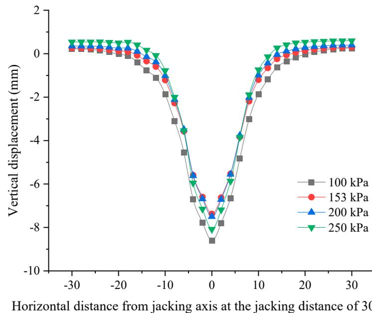
**Figure 16.** Vertical displacements of ground surface at the jacking distance of 30 m (the cross-section  $y = 30$  m) with the horizontal distance from jacking axis under different earth chamber pressures.
