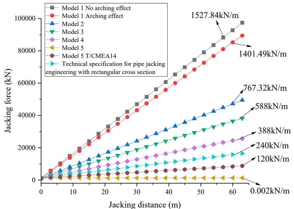
**Figure 9.** Jacking force prediction with distance under different models.
