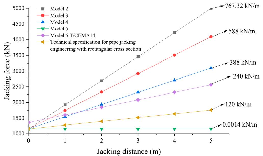
Figure 10. Partially enlarged detail of jacking force prediction with distance under different models.
