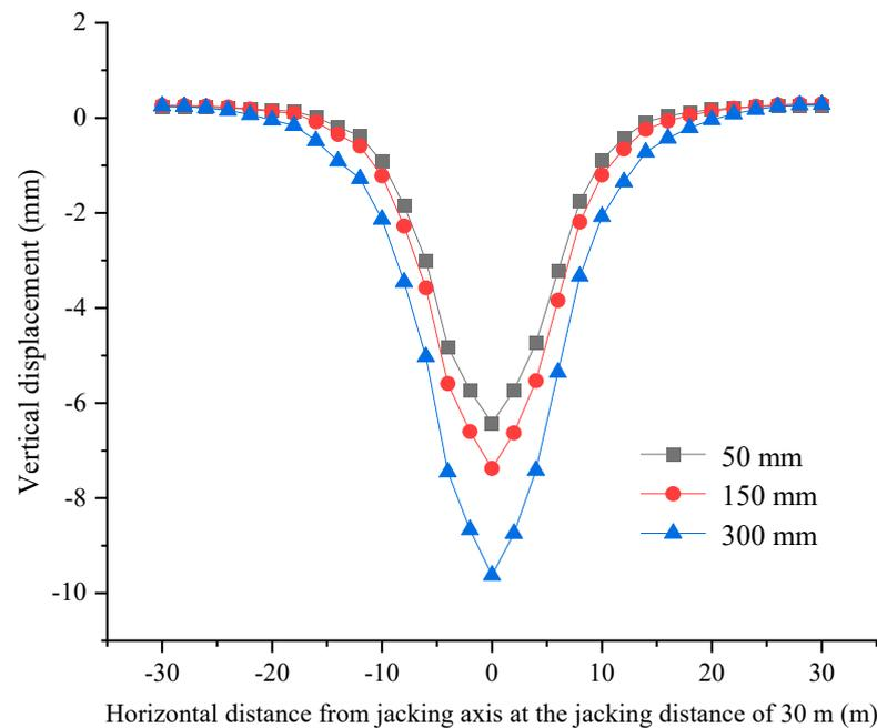
**Figure 12.** Vertical displacements of ground surface at the jacking distance of 30 m (the cross-section  $y = 30 \text{ m}$ ) under different slurry sleeve thicknesses after finishing jacking.
