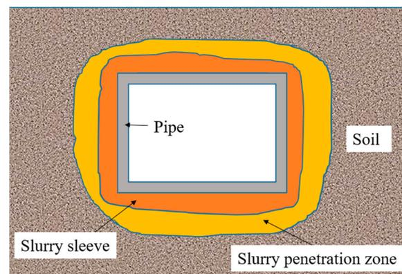
**Figure 8.** Full contact pipe–slurry interaction.
