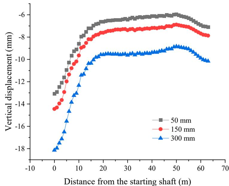
**Figure 13.** Vertical displacements of ground surface above the jacking axis under different slurry sleeve thicknesses after finishing jacking.
