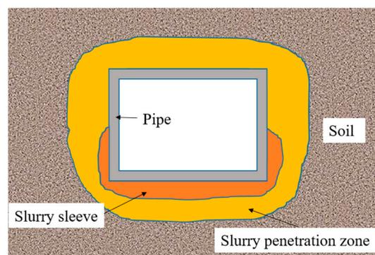
**Figure 6.** Pipe–slurry interaction at the bottom and 1/2 of both sides.
