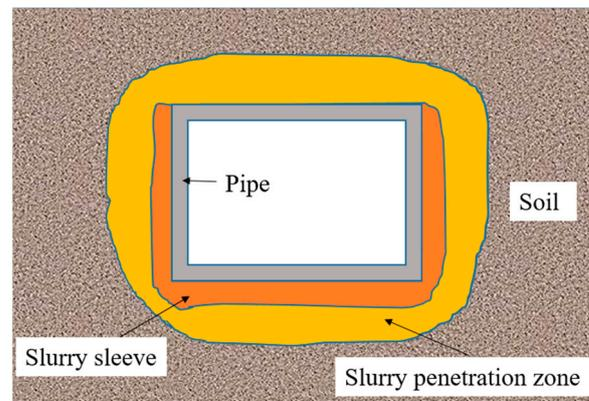
Figure 7. Pipe–slurry interaction at the bottom and both sides.
