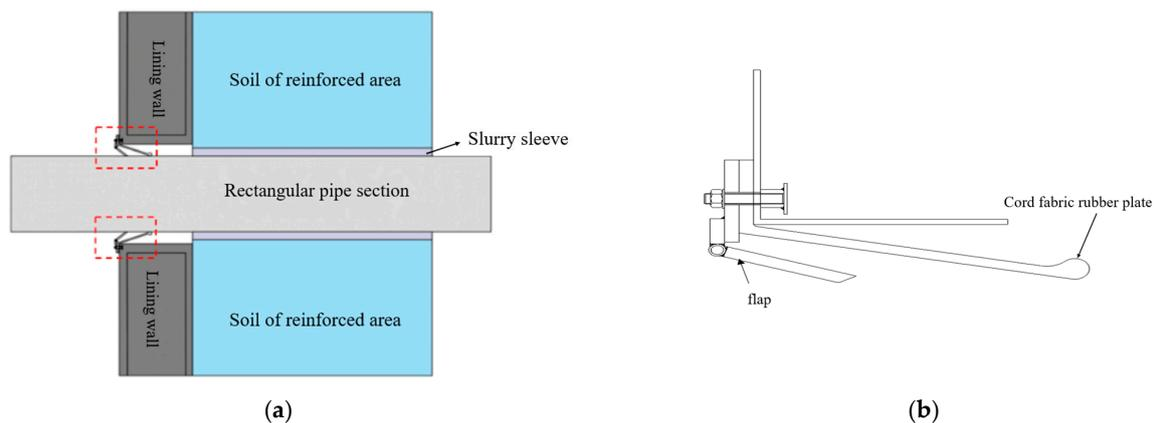
**Figure 18.** Installing waterproof rubber curtain for the tunnel portal: (a) longitudinal section of the waterproof device; (b) details of the waterproof device.
