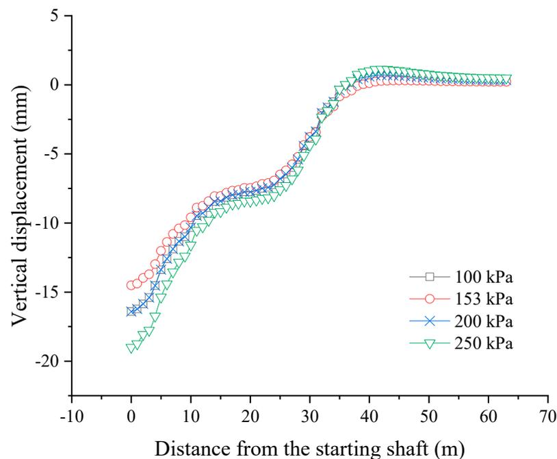
**Figure 17.** Vertical displacement of ground surface above the jacking axis under different earth chamber pressures when the tunneling distance is 30 m.
