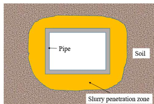
**Figure 3.** Full pipe–soil contact model.
