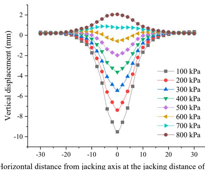
**Figure 14.** Vertical displacements of ground surface at the jacking distance of 30 m (the cross-section  $y = 30$  m) with the horizontal distance from jacking axis varying under different grouting pressures after finishing jacking.
