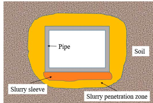
**Figure 5.** Pipe–slurry interaction at the bottom.
