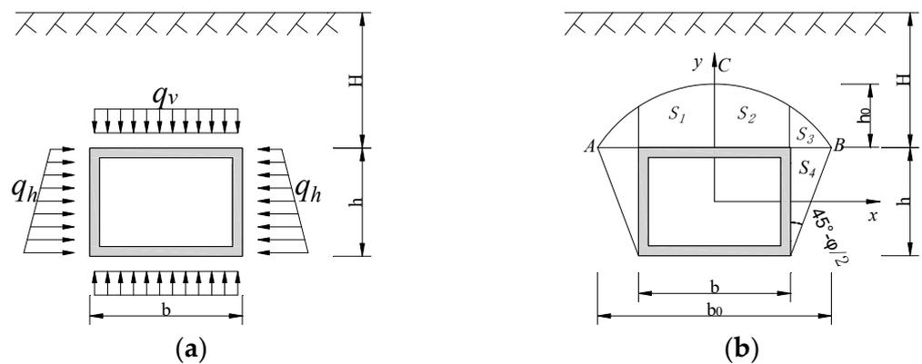
Figure 4. Stress diagram of full pipe–soil contact: (a) no arching effect; (b) arching effect.
