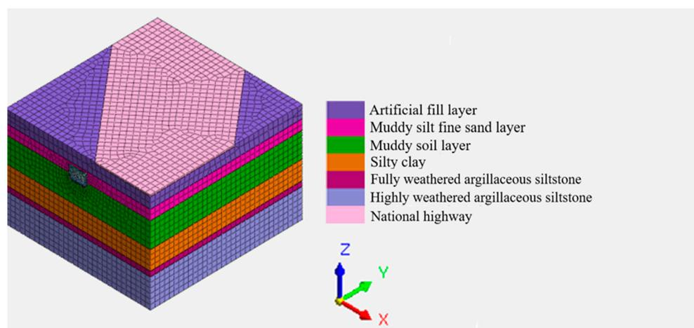
Figure 11. Numerical simulation model.
