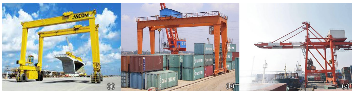
Figure 2. Examples of rubber tyred gantry crane (a), rail-mounted gantry crane (b), gantry crane (c).
