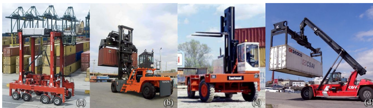
Figure 1. Examples of straddle carrier (a), fork lift (b), side loader (c), reach stacker (d).
