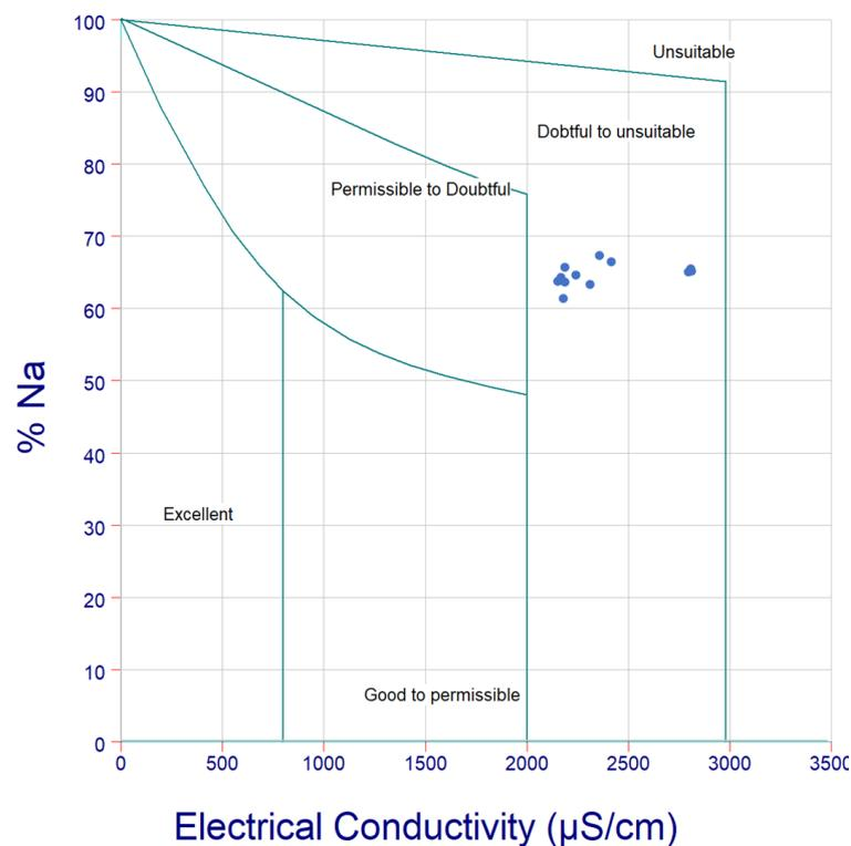
Figure 7. Water samples Suitability for Irrigation depicted by Wilcox Diagram.
