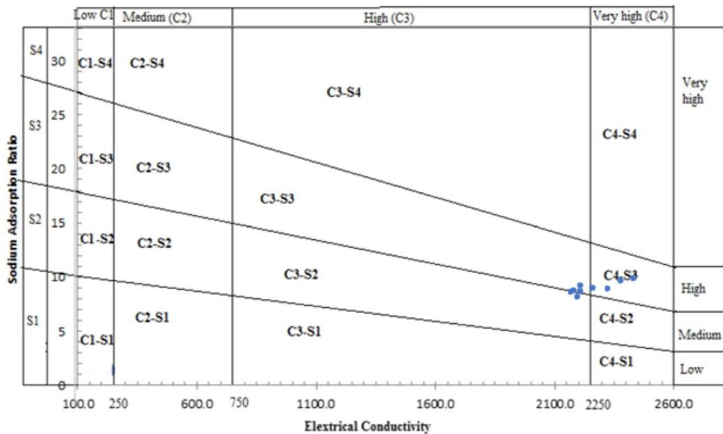
Figure 6. Classification of irrigation water suitability using USSS diagram based on SAR and EC according to Richards.
