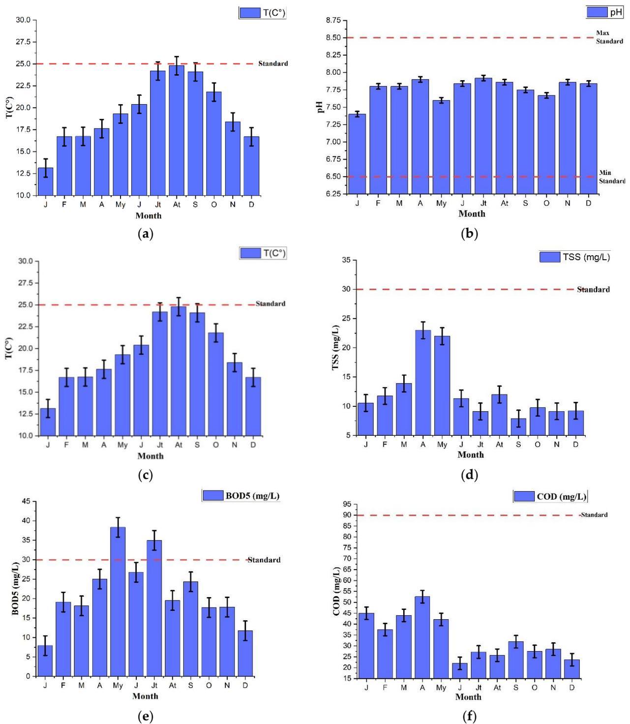
**Figure 4.** Monthly variation of physicochemical parameters at the outlet of the WWTP of Ain Sefra. ((a): temperature, (b): pH, (c): EC, (d): TSS, (e): BOD<sub>5</sub>, (f): COD).
