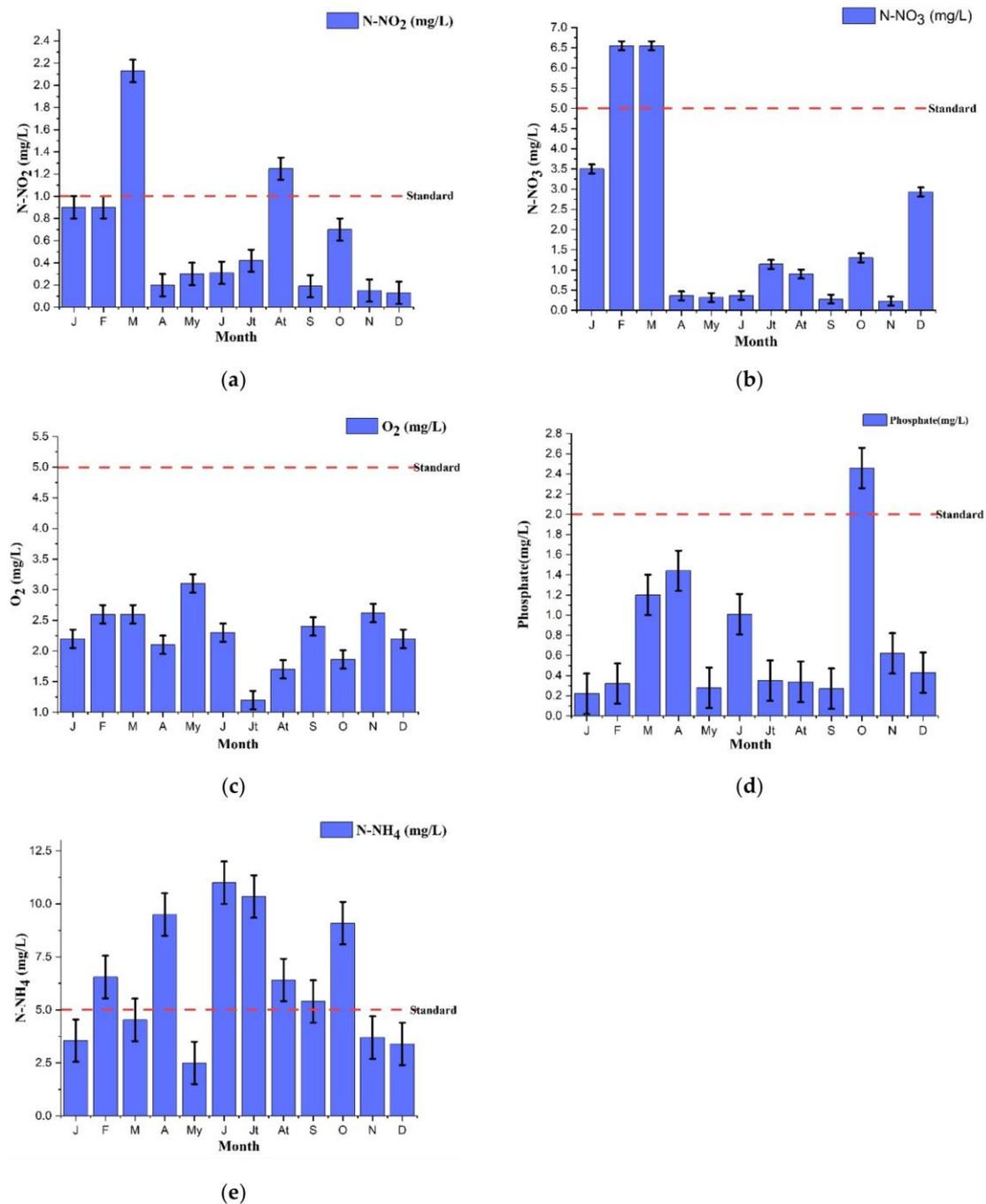
**Figure 5.** Monthly variation of physicochemical parameters at the outlet of the WWTP of Ain Sefra. ((a): N-NO<sub>2</sub>, (b): N-NO<sub>3</sub>, (c): DO, (d): PO<sub>4</sub>, (e): N-NH<sub>4</sub>).
