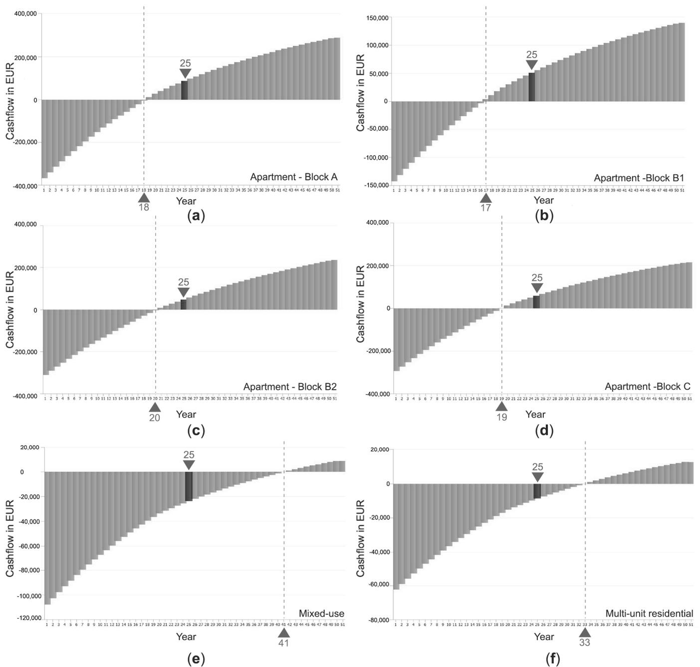
**Figure 10.** EU BIPV BOOST-based costing scenario NPV for the service life period of four apartment clusters (a–d), mixed-use (e), and multi-unit residential (f) buildings. Darker markings indicate discounted cash flow at 25 years of service life.
