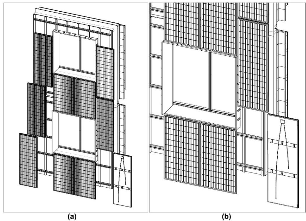
**Figure 3.** Overview (a) of the mounting system for BIPV façade modules on two prefabricated façade components of the building renovation system with finally positioned modules, modules before mounting on horizontal rails (two modules on the bottom left), and module back elevation with illustration of connection anchors, electricity connectors, and cabling (module on the bottom right), and detailed illustration (b).
