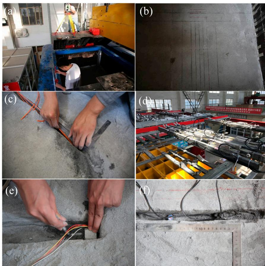
**Figure 6.** The main steps to install the sensors. (a) Position by total station. (b) Determine the outline of the caves. (c) Install the displacement sensors. (d) Install the grating ruler connected to the displacement sensors. (e) Install the strain brick. (f) Install the pressure cell.
