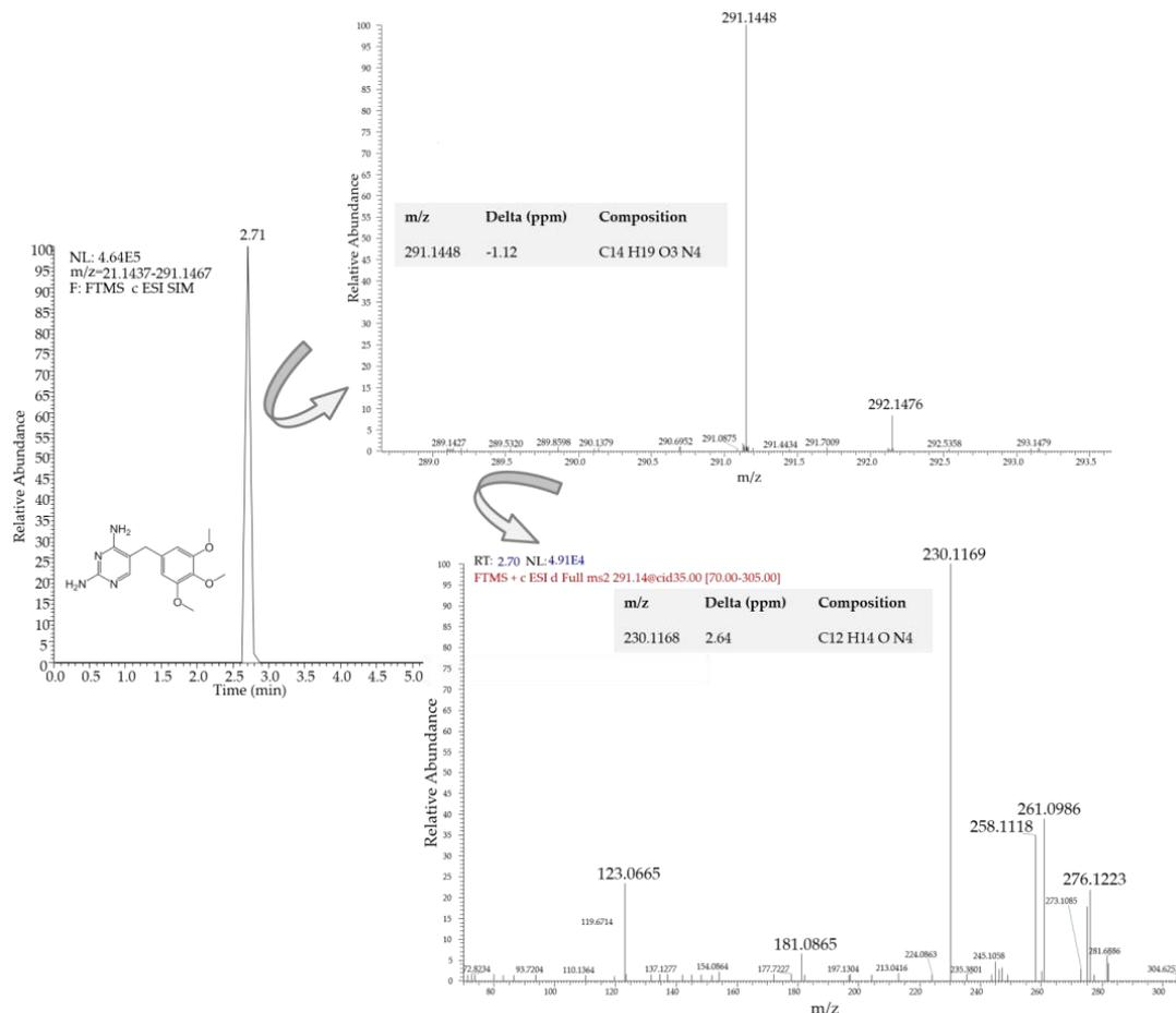
**Figure 5.** LC-LTQ/Orbitrap MS<sup>2</sup> extracted ion chromatogram (EIC) of seawater (S1e) containing trimethoprim at  $16.3 \text{ ng L}^{-1}$ .
