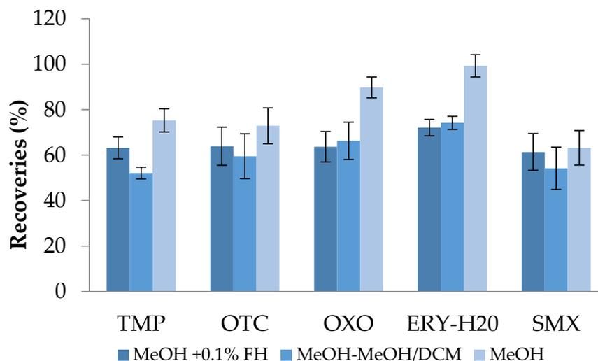
**Figure 3.** Antibiotics' recoveries (%) after distilled water extraction using SPE testing of different elution solvent systems (HLB cartridges; pH 3.5).
