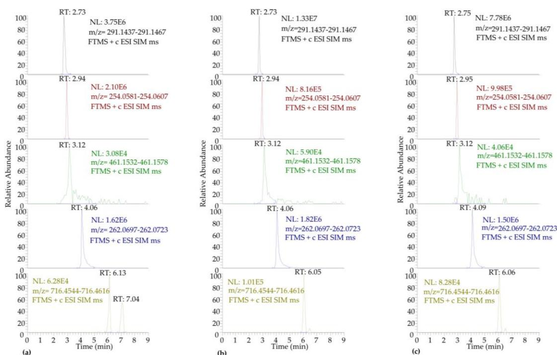
**Figure 1.** Comparative depiction of the SIM-LC-LTQ/Orbitrap MS chromatograms of the antibiotics in PI at concentration  $50 \mu\text{g L}^{-1}$ : (a) injection volume  $10 \mu\text{L}$ ,  $\text{AGC } 5 \times 10^5$ , 0.3% FH; (b) injection volume  $10 \mu\text{L}$ ,  $\text{AGC } 5 \times 10^4$ , 0.3% FH; (c) injection volume  $10 \mu\text{L}$ ,  $\text{AGC } 5 \times 10^4$ , no FH.
