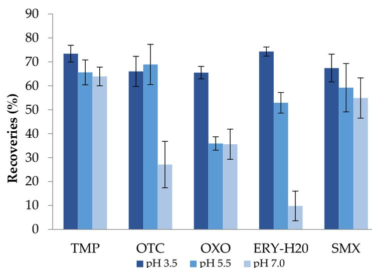
**Figure 2.** Recoveries (%) after SPE of the selected antibiotics in different pH conditions (HLB cartridges; methanol as the elution solvent).
