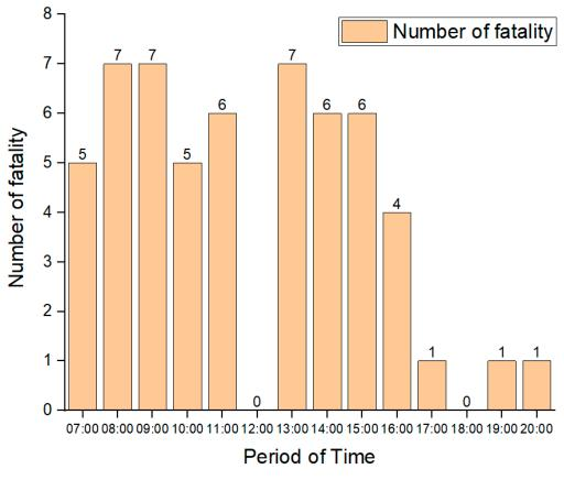
Figure 3. Analysis of the occurrence time of mobile crane accidents.
