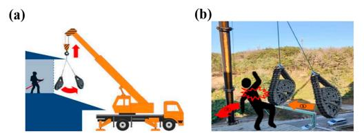
**Figure 6.** Hitting objects accident from mobile crane. (**a**) Schematic diagram of work at the time of the disaster and (**b**) schematic diagram of the situation at the time of the disaster.
