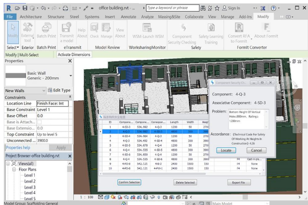
Figure 15. Visualization of the checking result.
