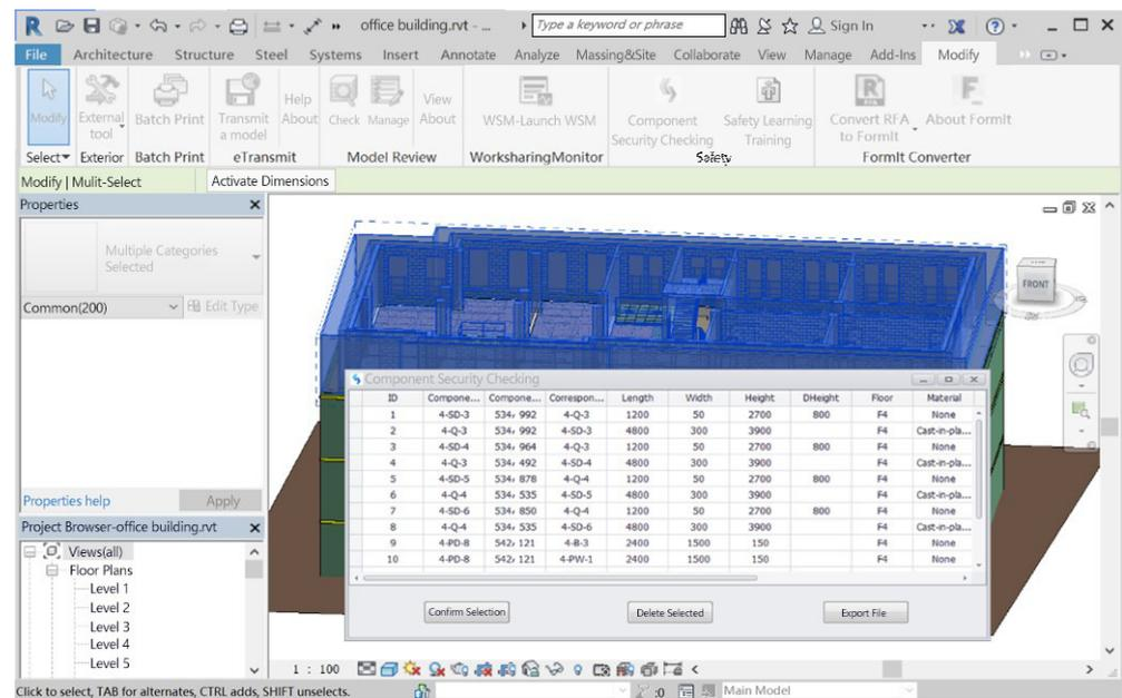
Figure 14. Safety checking results.
