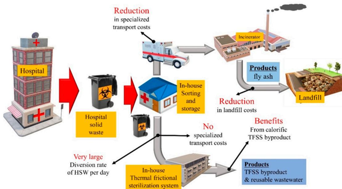
**Figure 1.** Conceptual framework for incineration–TFS integration system.
