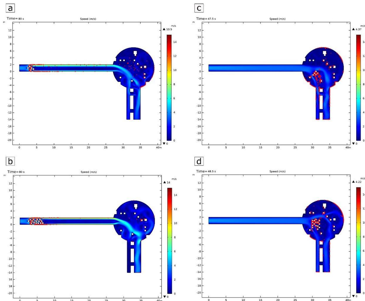
**Figure 5.** Simulations based on an articulated geometry, rebuilding the large circular room of the Pertosa-Auletta Cave, adding several discontinuities (white squares) and the tracking of massive particles (red circles), where the Y-axis represents the airflow speed (m/s) and the X-axis the linear dimension (m). In particular, a group of 5 (a,c) and 15 visitors (b,d) (white circles), positioned at the beginning of the long conduct (a,b) and in the large room (c,d), have been considered.
