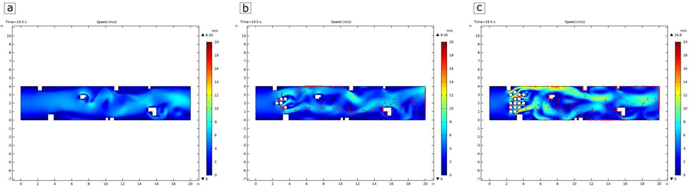
**Figure 3.** Simulations based on a simplified geometry of a linear conduct of the Pertosa-Auletta Cave, adding several discontinuities (white squares), where the Y-axis represents the airflow speed (m/s) and the X-axis the cylinder dimension (m). In particular, the basic physical model behavior (a) and the tracking of massive particles (red circles), considering a group of 5 (b) and 15 (c) visitors (white circles), are reported.
