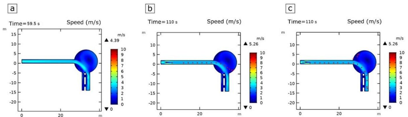
**Figure 4.** Simulations based on an articulated geometry, rebuilding the large circular room of the Pertosa-Auletta Cave, where the Y-axis represents the airflow speed (m/s) and the X-axis the linear dimension (m). In particular, the basic physical model behavior (a), the tracking of massive particles (red circles) from a discontinuity (white circle) (b), and the addition of heavier massive particles (c) are reported.
