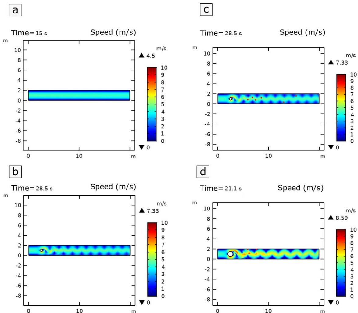
**Figure 2.** Simulations based on a simplified geometry of a linear conduct of the Pertosa-Auletta Cave, where the Y-axis represents the airflow speed (m/s) and the X-axis the cylinder dimension (m); in particular, the basic physical model behavior (a), with the addition of a discontinuity (white circle) (b), of the tracking of massive particles (red circles) (c) and of a larger discontinuity (white circle) (d) are reported.
