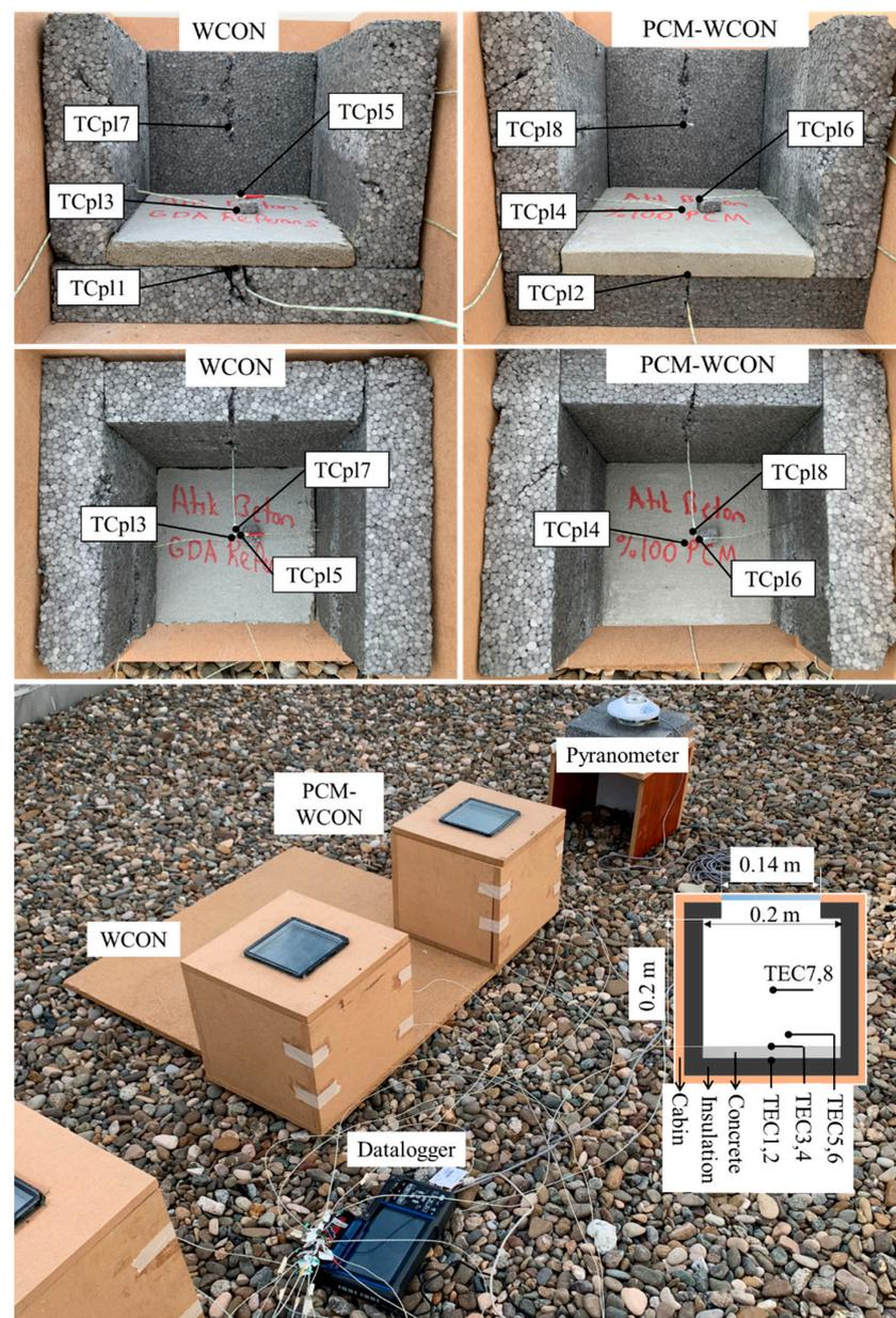
Figure 4. Experimental setup and thermocouple positions on the test cabins (28 April 2022).
