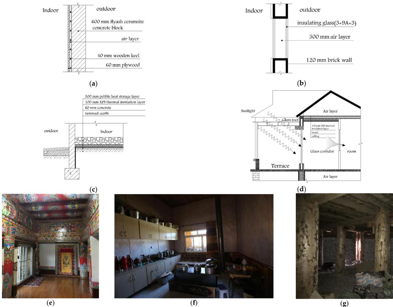
**Figure 3.** (a) “Composite wall” structure; (b) “double-window” structure; (c) “heat storage layer” structure; (d) “sunshine room” structure; (e) glass corridor; (f) kitchen; (g) storage room.
