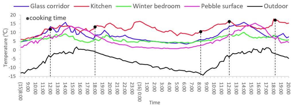
**Figure 6.** The air temperature change curve of test points.
