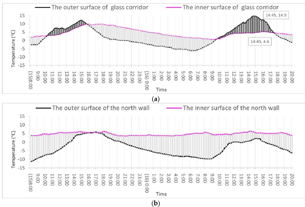
**Figure 8.** Changes in surface temperatures of enclosure materials: (a) glass corridor; (b) winter room.
