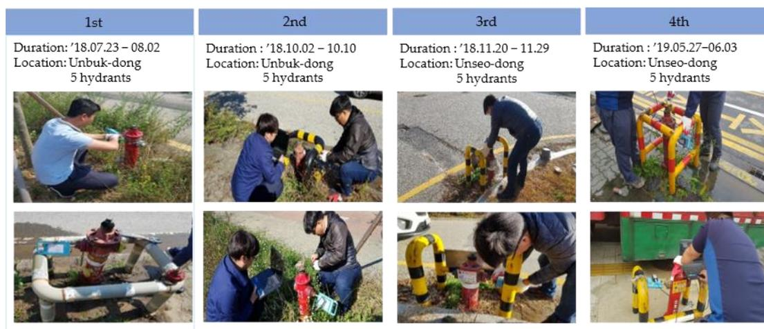
**Figure 19.** Measurement of actual water pressure in fire hydrants using a portable water pressure meter.
