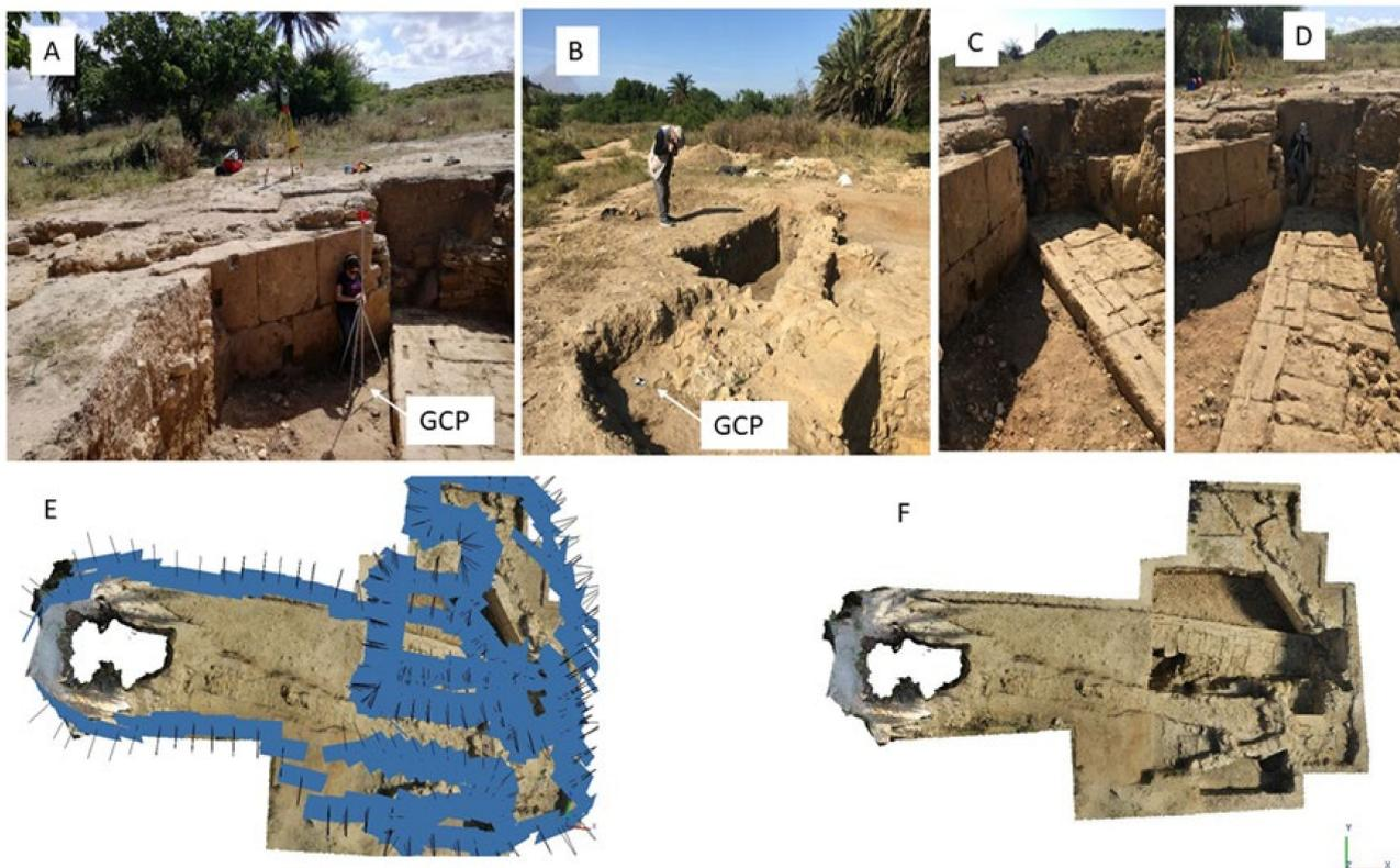
**Figure 17.** Photogrammetry for the archaeological excavation site in the city of Utica (Tunisia). (A) The survey of control points with total station; (B–D) the recording of photographs with a conventional camera from different points of view; (E) the points of view of all the photographs taken; (F) the final 3D model obtained.
