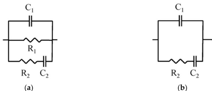
**Figure 2.** (a) Equivalent circuit used for fitting the impedance spectra obtained using the contacting method. (b) Equivalent circuit used for fitting the impedance spectra obtained using the non-contacting method.
