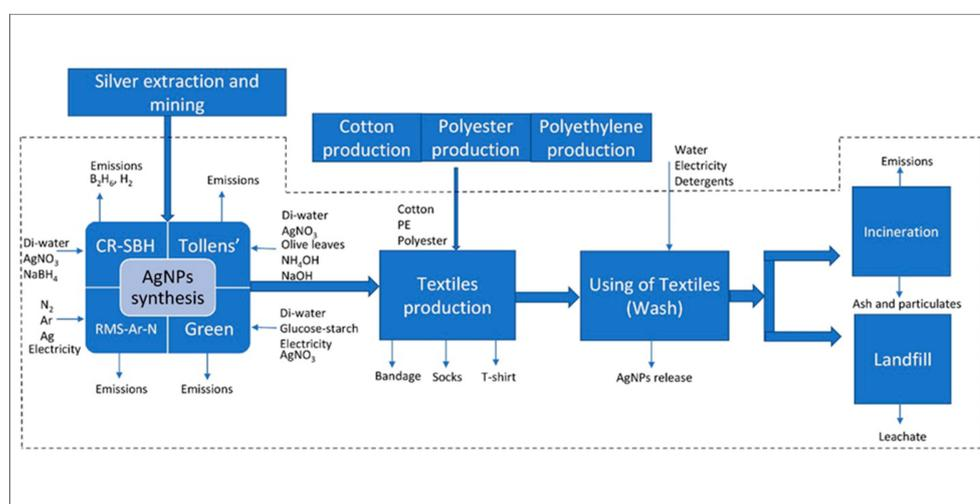
**Figure 1.** System boundary of various stages of silver nanoparticle (AgNP) life cycle.
