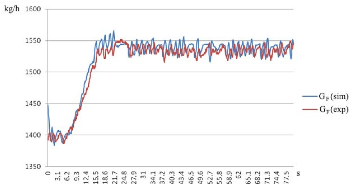
Figure 17. Dependence of the fuel consumption on the time of the transient process during the step increase load (red line—experimental, blue line—model).
