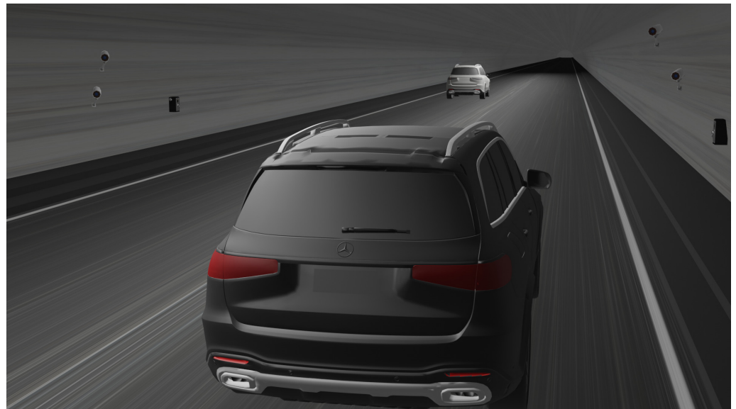
Figure 1. Proposed solution for placement of IP cameras and thermal cameras in two-lane tunnel. Height of IP cameras is approximately 1580 mm and 2110 mm and cameras are facing cars at an angle of 20^\circ with respect to the walls of the tunnel; in case of thermal camera, proposed height is 1230 mm, and camera is facing perpendicular to the road.
