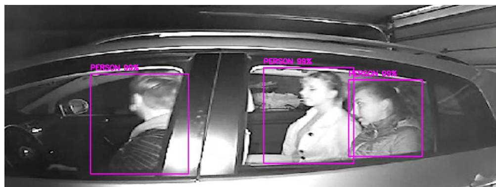
Figure 9. Result of passenger detection (including driver) using model based on modified YOLOv3.
