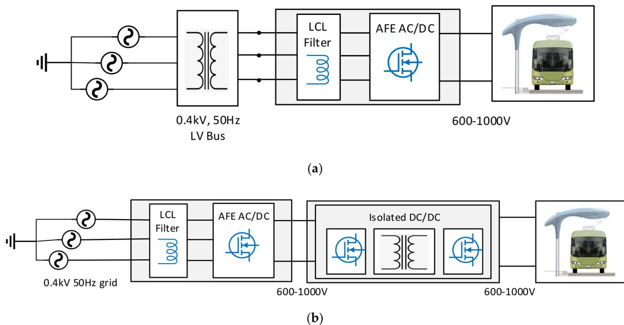
**Figure 5.** Topologies for BEB charging infrastructure with (a) LFT- and (b) HFT-based isolated DC/DC converter.
