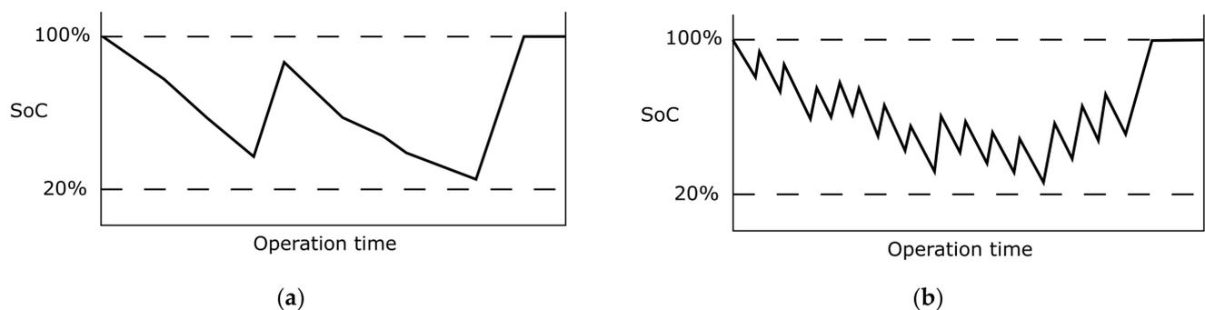
**Figure 4.** Typical SoC profile of a (a) depot charging BEB and (b) opportunity and dynamic wireless charging BEB.
