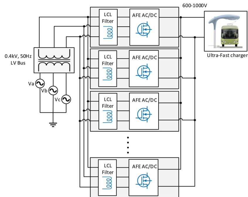
Figure 6. BEB charging infrastructure with LFT and modular PECs.
