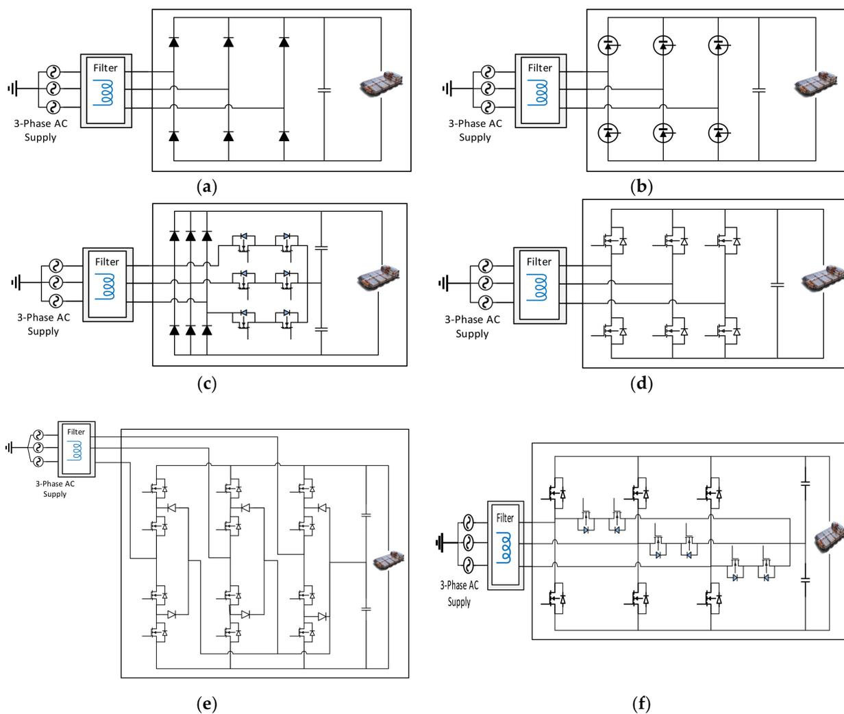
**Figure 8.** Three-phase AFE converter topologies; (a) Diode bridge rectifier, (b) thyristor bridge rectifier, (c) Vienna rectifier, (d) Two-level active front end rectifier, (e) Three-level NPC type converter, (f) Three-level T-type AFE converter.
