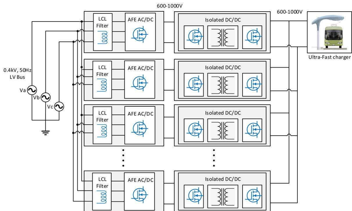
Figure 7. BEB charging infrastructure with HFT and modular PECs.
