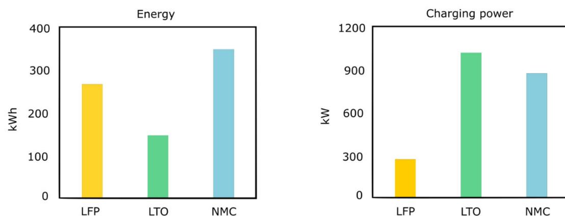
**Figure 2.** Battery capacity and maximum charging power of different lithium-ion battery types for a typical city BEB (adapted from [13]).
