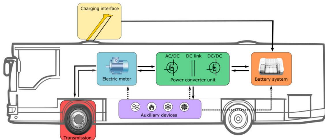
**Figure 1.** Powertrain topology of a battery electric bus.
