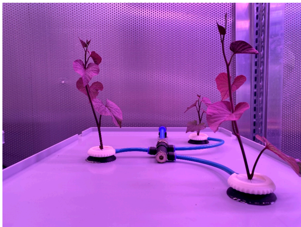
Figure 8. Newly developed aeroponic cultivation system for Ipomoea batatas in IVFs.
