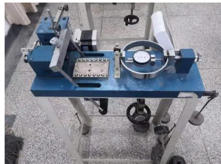
**Figure 2.** Electric strain-type direct shear apparatus.
