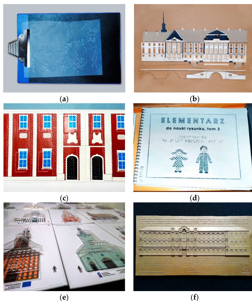
Figure 1. Various techniques and technologies of making typhlographics: (a) A simple drawing on tracing paper; (b) sticker made of various textures; (c) dotted drawing from a braille printer; (d) thermoprint; (e) “Braillon” made by thermoforming; (f) relief in metal. Photo by: (a,b,d,e) Kłopotowski, M.; (c) Magdziak, M.; (f) Jakubowski, M.; Figures edited by Magdziak, M.
