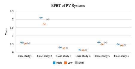
Figure 11. Energy payback time (EPBT) of PV systems varies based on maintenance energy investment.
