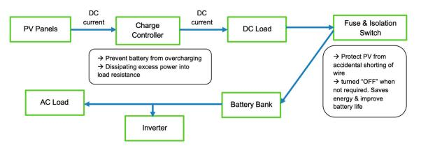
Figure 2. Solar standalone system balance-of-system (BOS).
