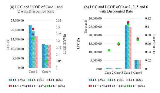
**Figure 14.** (**a**) Life cycle cost (LCC) and levelised cost of energy (LCOE) of case 1 and 4. (**b**) LCC and LCOE of case 2, 3, 5, and 6 based on different discount rates of 2%, 4%, and 6%.
