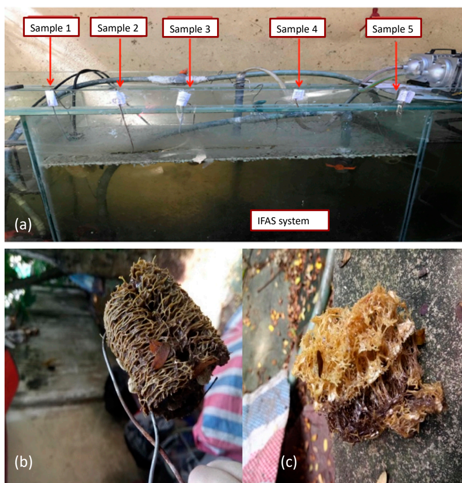
Figure 3. Evaluation of durability of loofah sponges in IFAS tank (a) the arrangement of 5 samples; (b) the sample 1 after 5 days; (c) the sample 3 after 30 days.
