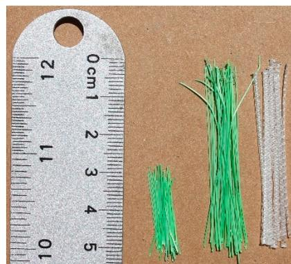
**Figure 2.** RPFs used in this study and Sika Fiber®Force PP-48 fibers.
