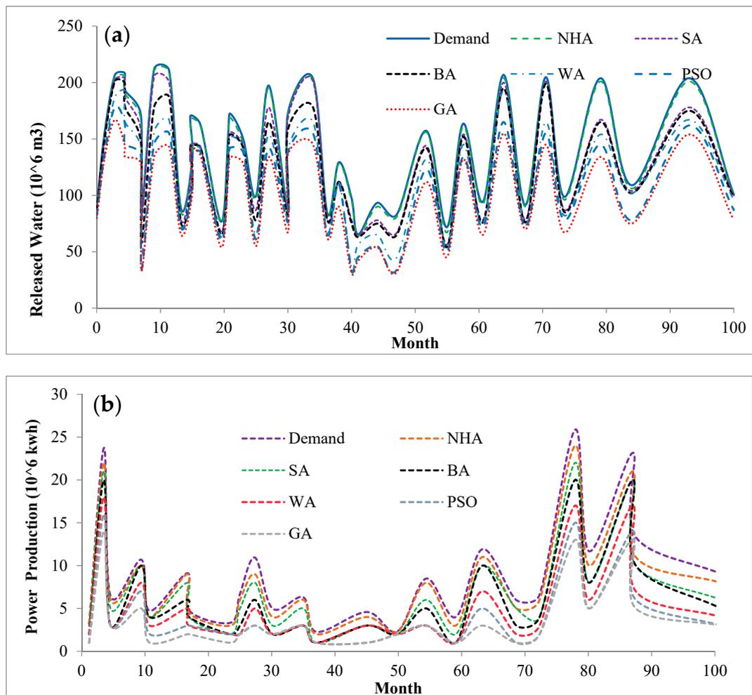
**Figure 9.** (a) Released water for downstream irrigation and (b) power production for downstream demand.
