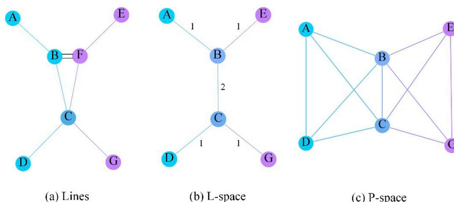
**Figure 1.** (a) A simple urban rail transit (URT) map with two lines. Stations A-G are serviced by Line 1 (blue) and Line 2 (purple), while B and F are separate stations with pedestrian connections between platforms; (b) L-space network; (c) P-space network.
