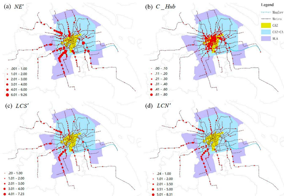
**Figure 10.** Vulnerability in terms of  $NE'$ ,  $LCS'$  and  $LCN'$  under a single node attack, compared with the  $C\_Hub$  of each node in the Shanghai URT network in 2020.
