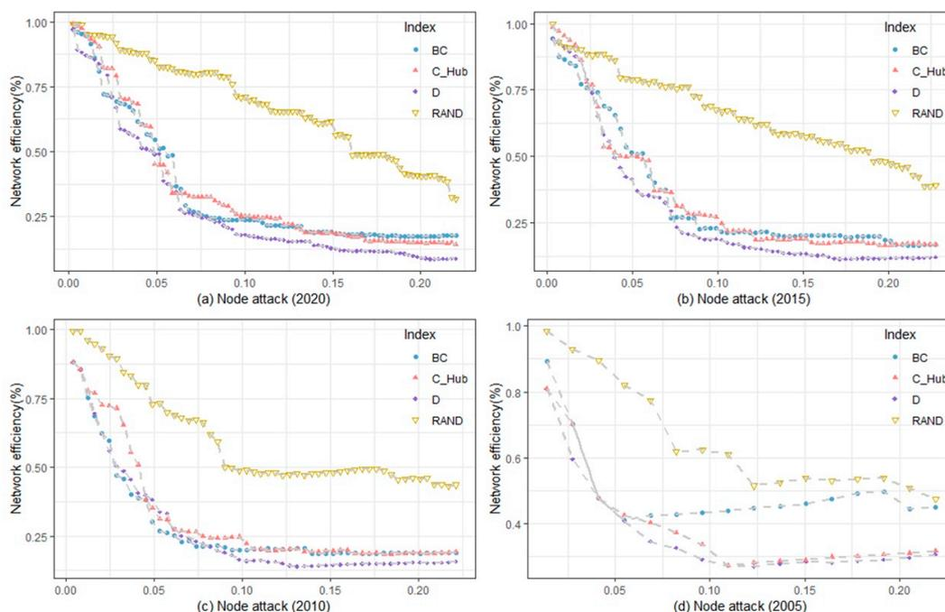
**Figure 5.** Damages of network efficiency under multiple nodes attacks in four stages.
