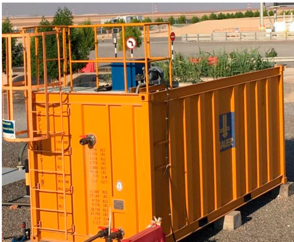
Figure 5. The compact, mobile aerated constructed wetland unit “ReedBox” [54] (Courtesy: Bauer Resources GmbH— https://www.bauer.de/bre ).
