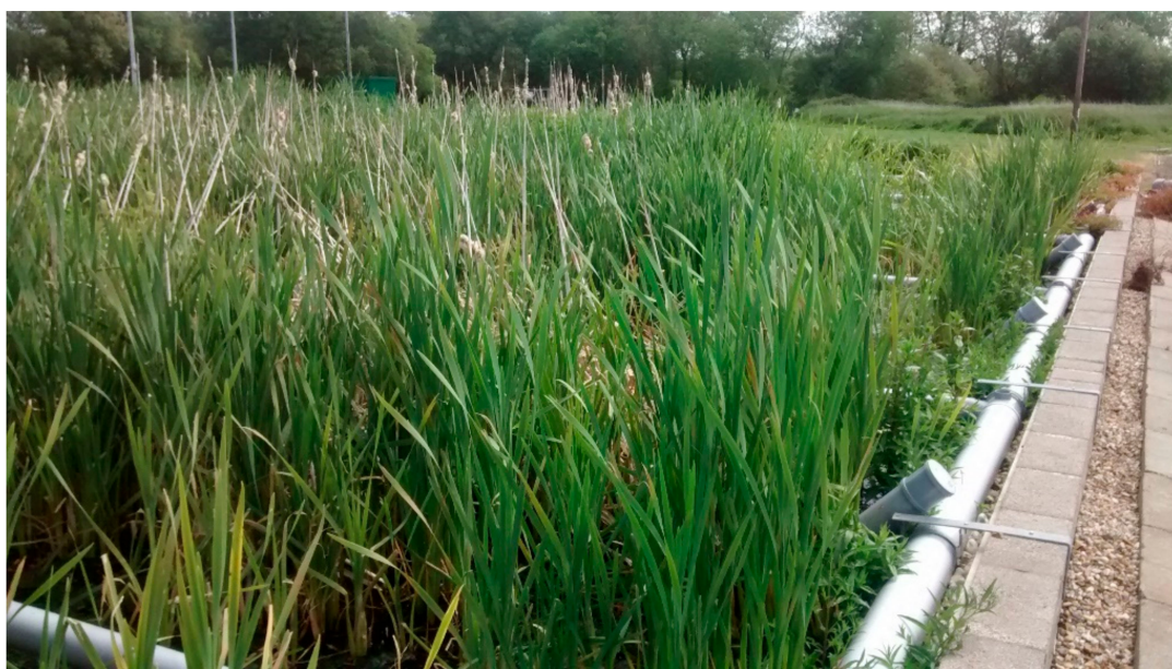
Figure 4. Aerated constructed wetland at Petersfield sewage treatment works, Hampshire, UK [45].
