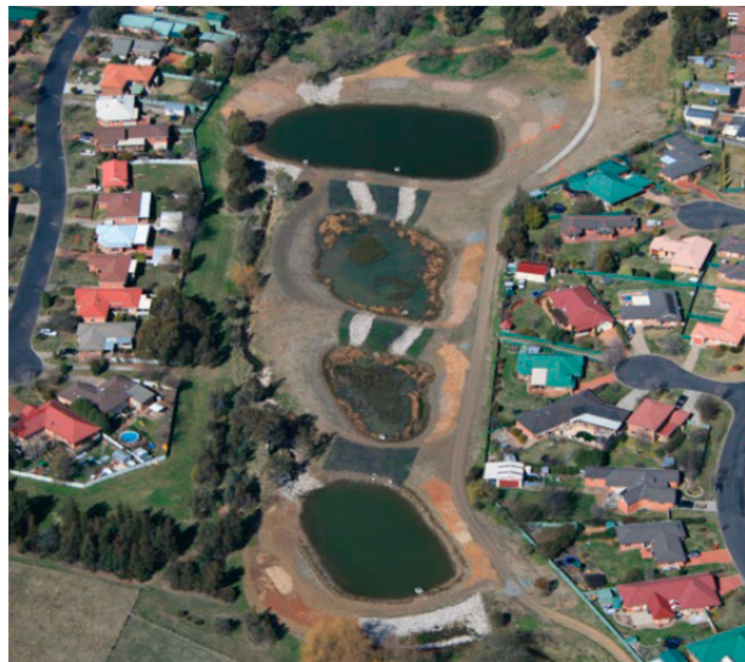
Figure 8. The constructed wetland at the Somerset Park, Orange, New South Wales, Australia that collects and treats stormwater [82].
