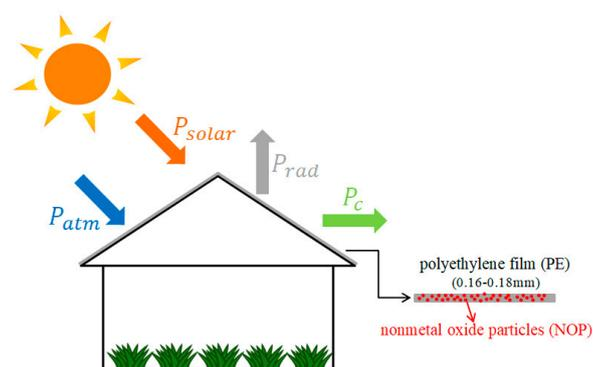
**Figure 1.** A schematic indicating the heat fluxes for a greenhouse.
