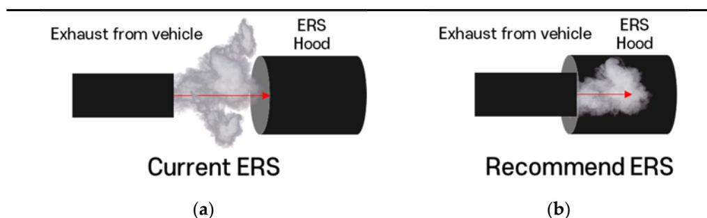
**Figure 4.** Schematic diagram of ERS: (a) current ERS and (b) recommend ERS.
