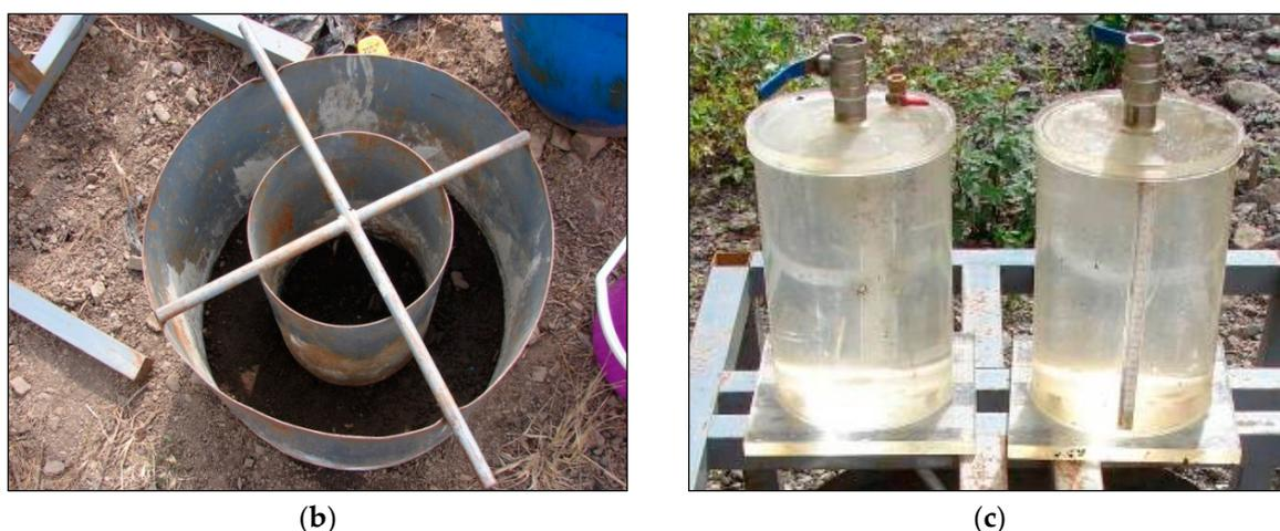
**Figure 6.** The adopted double rings infiltration test. (a) Schematic layout of double rings infiltration test. (b) Photo of double ring instrument. (c) Photo of Mariotte's bottle.
