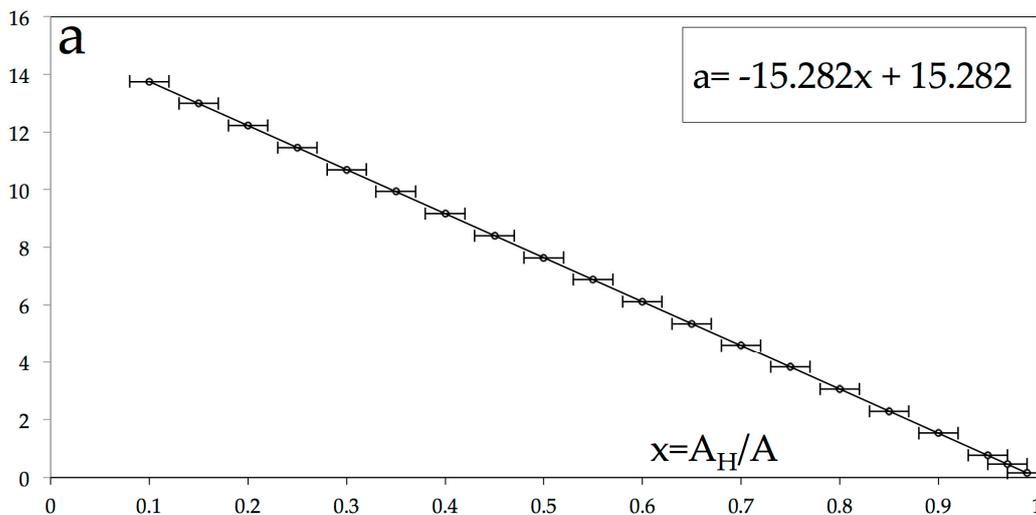
**Figure 6.** The effect of the area ratio  $x = A_H/A$  to the coefficient  $a$  in Equation (20). The error bars show the displacement of the line when the reflectance in the infrared region varies from the given value by  $\pm 10\%$ .
