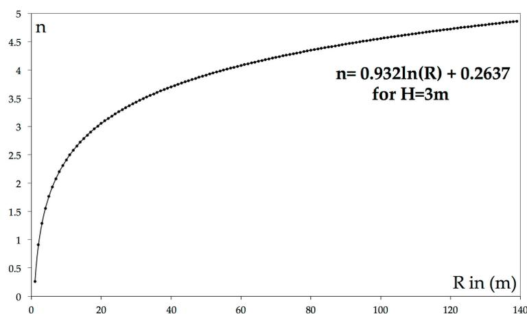
**Figure 7.** Effect of the radius of the sphere on the collector and radiator temperatures exponent  $n$  for a mixing length  $H = 3\text{ m}$ , and  $x = 0.1$ .
