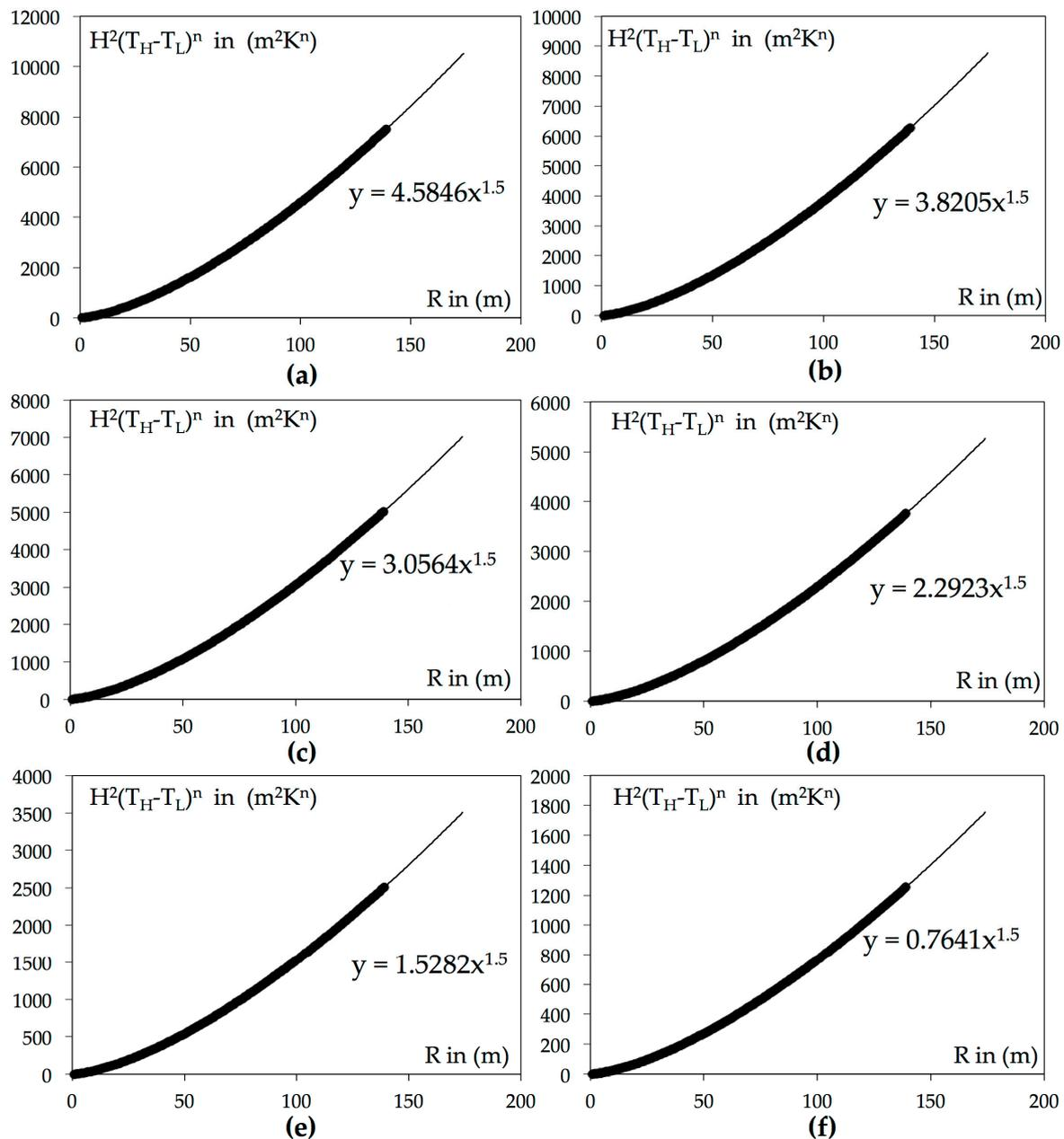
**Figure 4.**  $H^2(T_H - T_L)^n$  evolution for different values of  $x = A_H/A$  as the radius  $R$  of the spherical volume increases. We observe that  $H^2(T_H - T_L)^n$  evolution follows a pattern of  $y = ax^n$  where  $n = 3/2$ . Consequently, we can say that  $H^2(T_H - T_L)^n = aR^{3/2}$  whereas  $a$  evolves as  $x$  changes (a)  $x = 0.7$ ; (b)  $x = 0.75$ ; (c)  $x = 0.8$ ; (d)  $x = 0.85$ ; (e)  $x = 0.9$ ; (f)  $x = 0.95$ .
