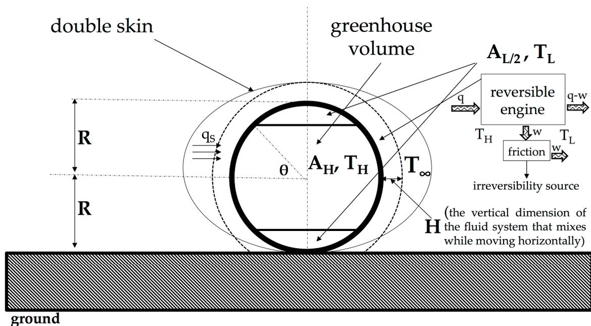
Figure 1. Urban greenhouse model equipped with a double skin envelope.
