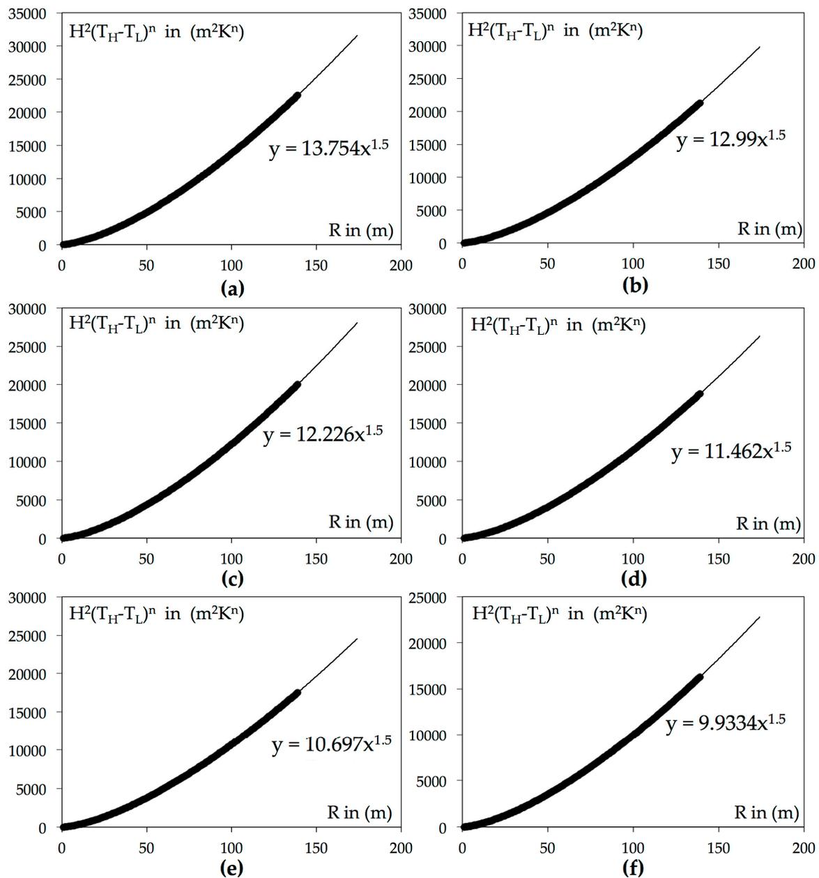
**Figure 2.**  $H^2(T_H - T_L)^n$  evolution for different values of  $x = A_H/A$  as the radius  $R$  of the spherical volume increases. We observe that  $H^2(T_H - T_L)^n$  evolution follows a pattern of  $y = ax^n$  where  $n = 3/2$ . Consequently we can say that  $H^2(T_H - T_L)^n = aR^{3/2}$  whereas  $a$  evolves as  $x$  changes (a)  $x = 0.1$ ; (b)  $x = 0.15$ ; (c)  $x = 0.2$ ; (d)  $x = 0.25$ ; (e)  $x = 0.3$ ; (f)  $x = 0.35$ .
