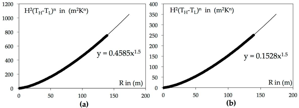
**Figure 5.**  $H^2(T_H-T_L)^n$  evolution for different values of  $x = A_H/A$  as the radius  $R$  of the spherical volume increases. We observe that  $H^2(T_H-T_L)^n$  evolution follows a pattern of  $y = ax^n$  where  $n = 3/2$ . Consequently, we can say that  $H^2(T_H-T_L)^n = aR^{3/2}$  whereas  $a$  evolves as  $x$  changes (a)  $x = 0.97$ ; (b)  $x = 0.99$ .
