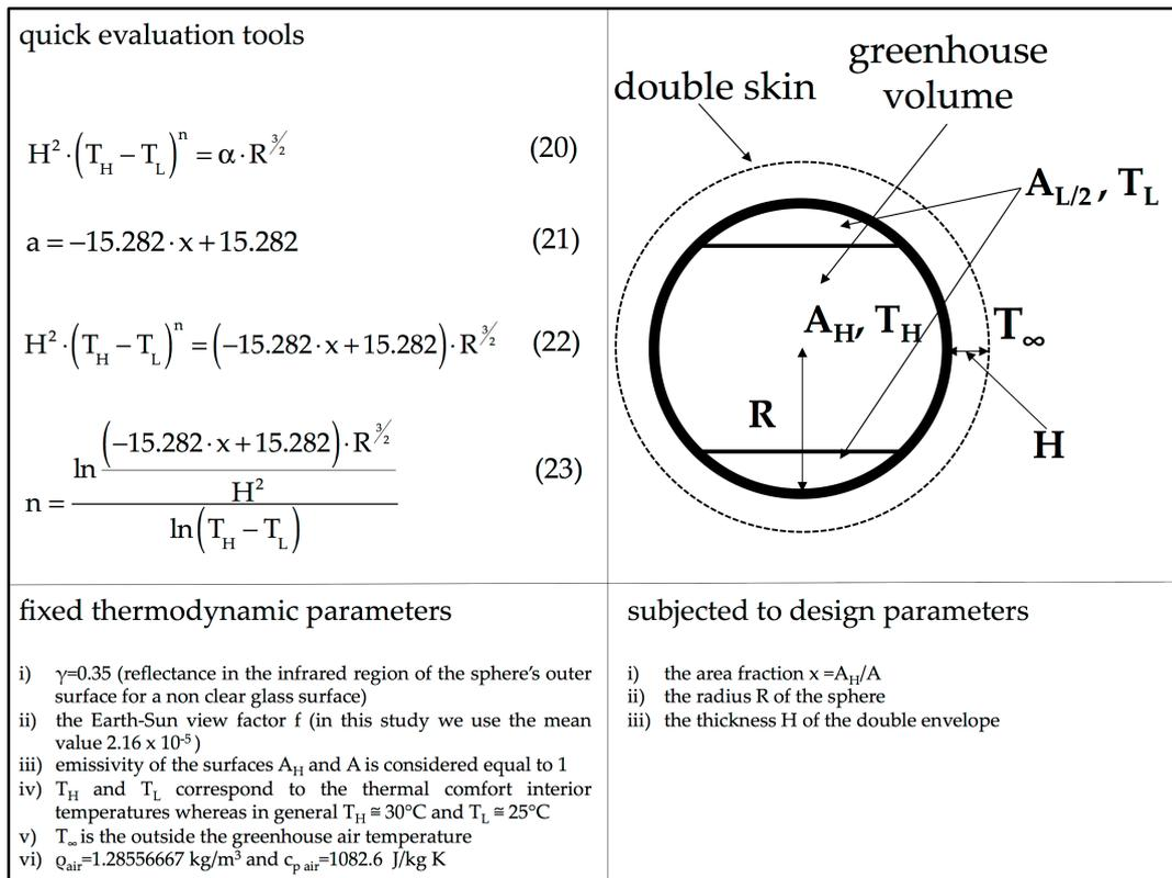
**Figure 8.** The quick evaluation tools based on the constructal law that the present paper proposes, the main geometry, the fixed thermodynamic parameters and the subjected to design parameters of the studied problem. The present paper aims at introducing a new methodology and approach that simplifies the calculation of the main thermodynamic behavior of a spherical urban greenhouse.
