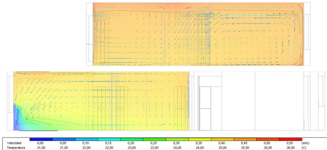
Figure 12. Simulated (CFD) of the house's thermal behaviour; 1 August 2018, 3 pm.
