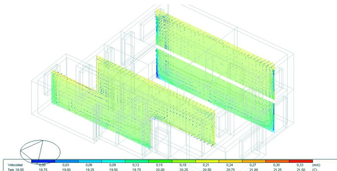
Figure 11. Simulated (CFD) of the house's thermal behaviour; 1 February 2019, 9 am.
