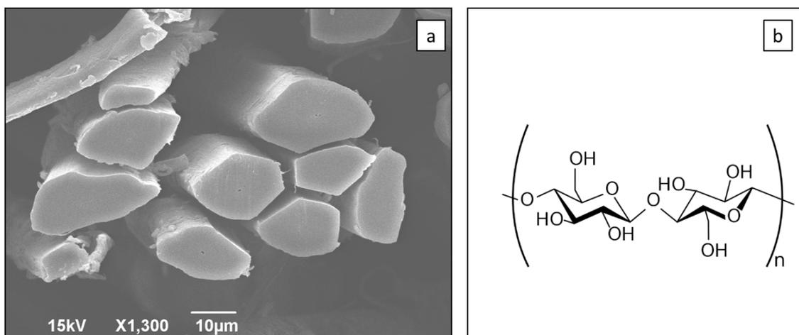
**Figure 1.** (a) Scanning Electron Microscopic image of cross section of bundle of flax fiber, (b) repeating unit of cellulose.
