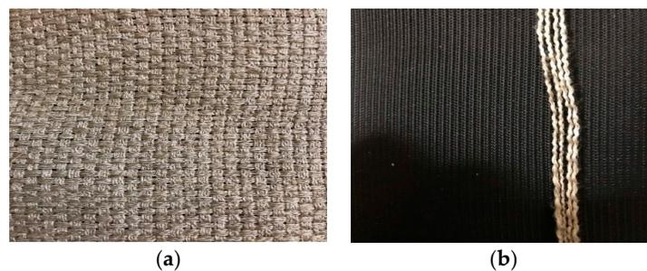
**Figure 3.** (a) Woven mat of the flax fibers (plain weave), (b) flax fiber tow pulled out of the weave.
