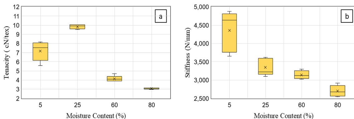
Figure 7. (a) Distribution of tenacity for various tow moisture levels, (b) distribution of stiffness for various tow moisture levels.
