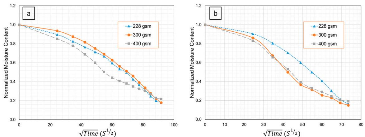
**Figure 5.** Desorption curves for moisture through non-woven random flax fiber mats for different areal densities: (a) at 55°C, (b) at 80 °C.
