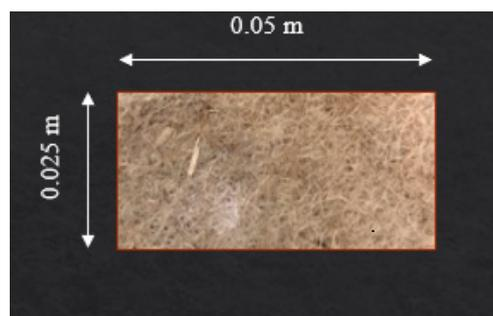
**Figure 2.** Non-woven flax fiber mat cut to size before the immersion into distilled water.
