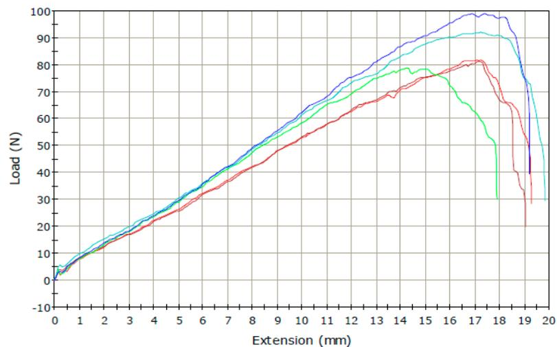
Figure 6. Typical load-displacement curve for flax fiber tow.
