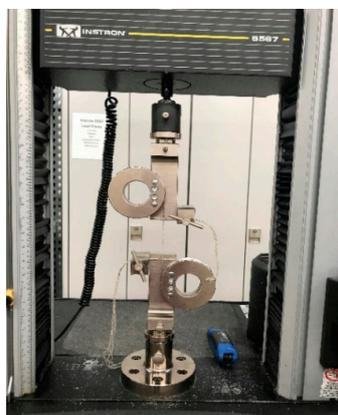
**Figure 4.** Flax fiber tows in filament grips of the Instron 5567 universal testing machine.
