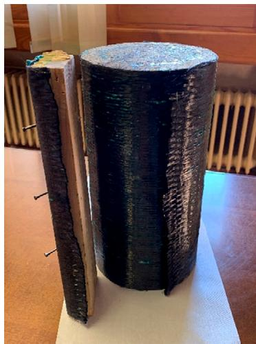
**Figure 5.** Final view of the specimen reinforced with initial tension.
