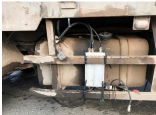
**Figure 2.** Diesel consumption instrument.
