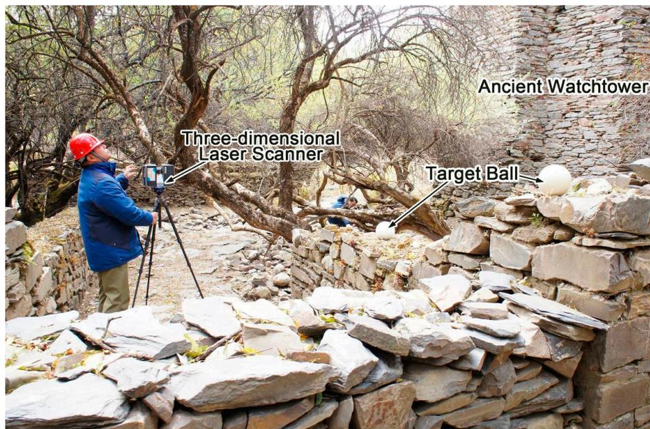
**Figure 8.** 3D laser scanning outside the watchtower.
