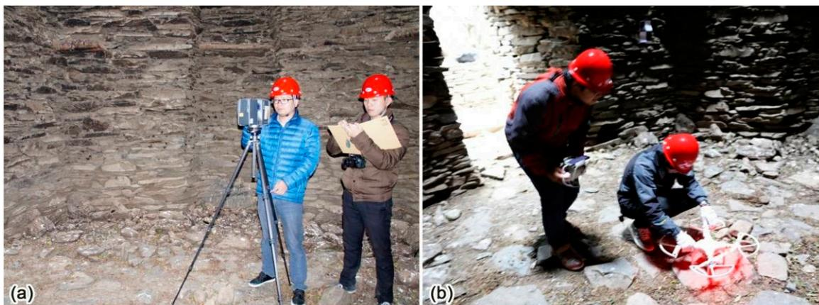
**Figure 9.** (a) 3D laser scanning inside the watchtower, (b) manipulation of the unmanned aerial vehicle inside the watchtower.
