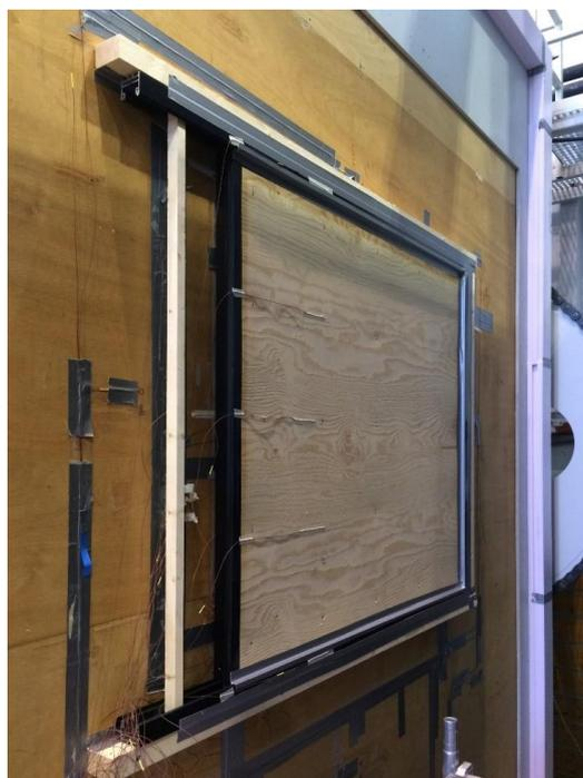
**Figure 6.** The shutter system in the hot box. The photo shows test case “3 tapes”.
