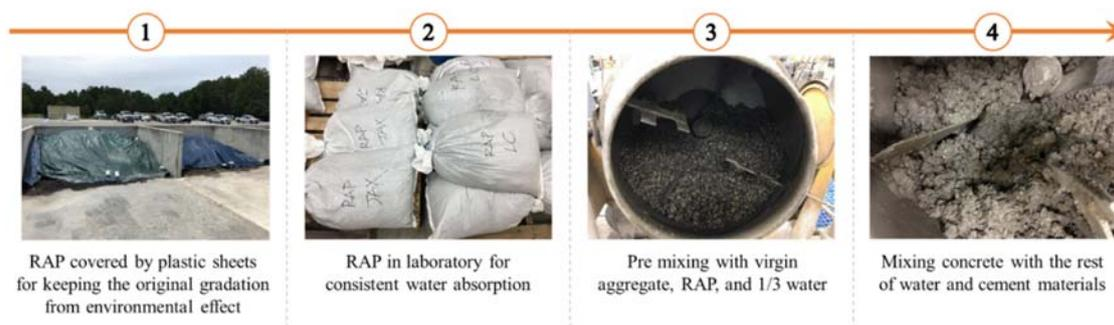
**Figure 1.** Preparation of RAP and process of concrete mixing.
