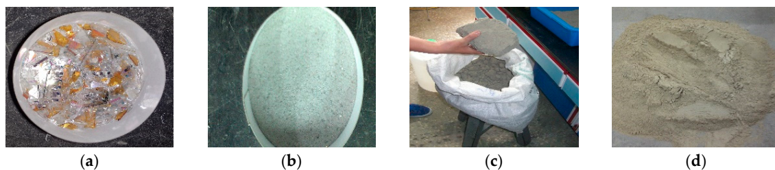
Figure 1. Raw materials. (a) Original thin-film transition liquid crystal display (TFT-LCD) waste glass; (b) Refined TFT-LCD glass powder; (c) Original reservoir sediments; (d) Refined reservoir sediments.
