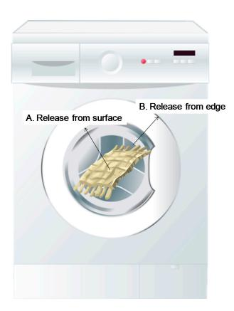
**Figure 1.** The microplastics can either shed from the surface of the fabric (A) or from the cut edge of the fabric (B).
