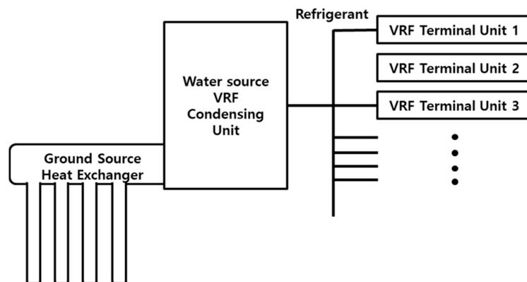
Figure 2. Typical components of ground-source variable refrigerant flow (VRF) system.
