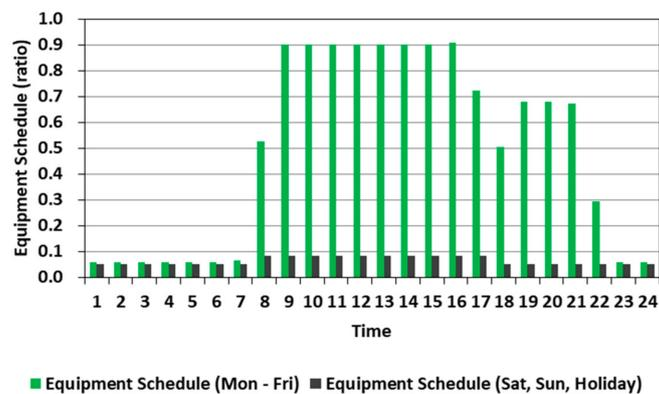
Figure 7. Equipment schedules used for the office-building model.
